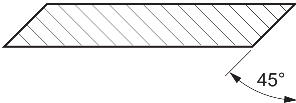
Figure 34 —Sharpen a rotor knife
