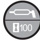
Look for this decal on your machine. It indicates a grease point and the interval in hours.
