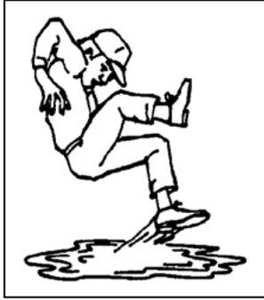
3. Make sure there is plenty of ventilation. Never operate the machine or the towing vehicle in a closed building. The exhaust fumes may cause asphyxiation.
