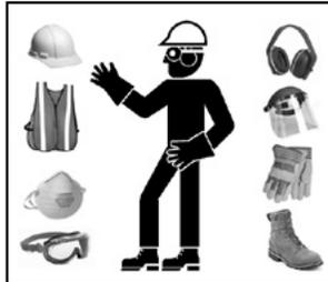
are recommended during assembly, installation, operation, adjustment, maintaining, repairing, removal, cleaning, or moving the chipper. Do not allow long hair, loose fitting clothing or jewellery to be around equipment.
