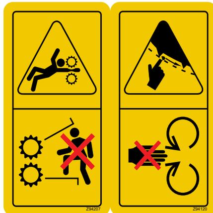
**Caution:** Do not reach or step into the feed hopper at any time, use a stick or branch to push any piece of material into the rollers that does not move on its own. If the jam persists then stop the engine and wait for the rotor to stop and then clear the jam. **Do not chance getting your hand or foot caught in the rollers.**
