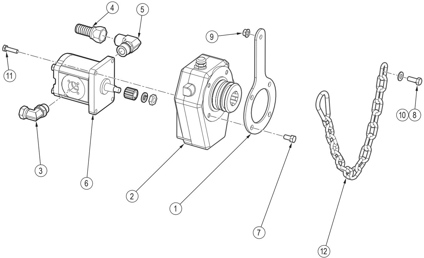
**Figure 1**—Gearbox and pump assembly components
