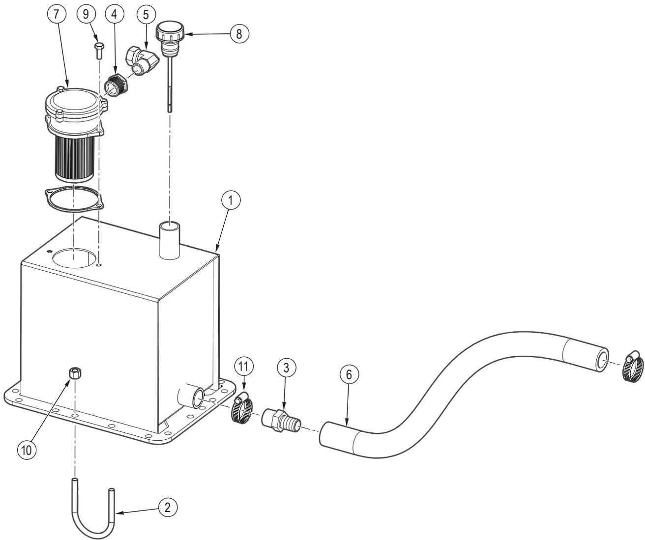
**Figure 2**—Hydraulic-fluid reservoir components
