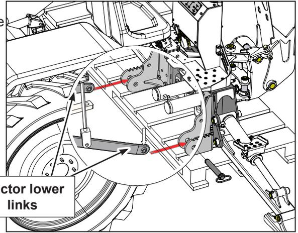
3. Find the centre tie back bushing (1" id) and check that it fits on the tractor's top link, if the bushing is too wide then it will have to be cut to fit.
