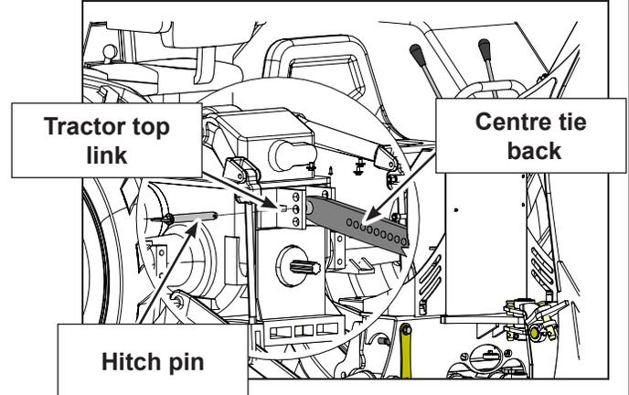
5. Assemble the two tie back bar sides to backhoe seat brace / top link with a bolt. (not included)
