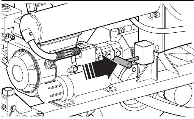
Fig. 29—Lock Pin Fully Engaged on WXR740 Series
