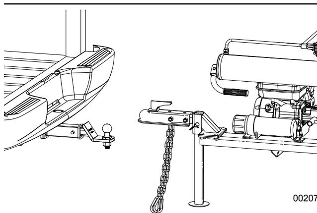
Fig. 31—Ball Hitch Aligned
