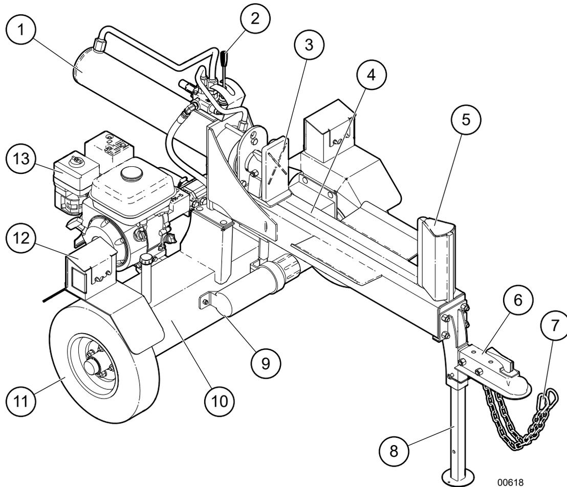
**Fig. 3**–WXR720, WXR720L Wood Splitter Components
