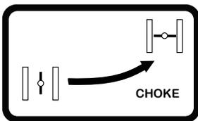
**Choke:** This left/right slider controls the position of the choke. Slide the choke to the right to close the choke for starting when the engine is cold. Slide the knob to the left to open the choke as the engine warms. Always slide the choke fully to the left when operating the machine.
