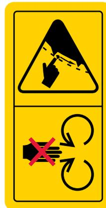
**Caution:** Do not reach into the feed hopper at any time, use a stick or branch to push any piece of material into the rollers that does not move on its own. If the jam persists then stop the engine and wait for the rotor to stop and then clear the jam.
