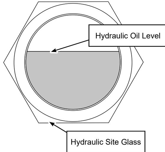
Hydraulic oil level should be checked daily, and the quality of the oil should be inspected every 50 hr. If the oil is dirty or smells burnt, it should be replaced.
