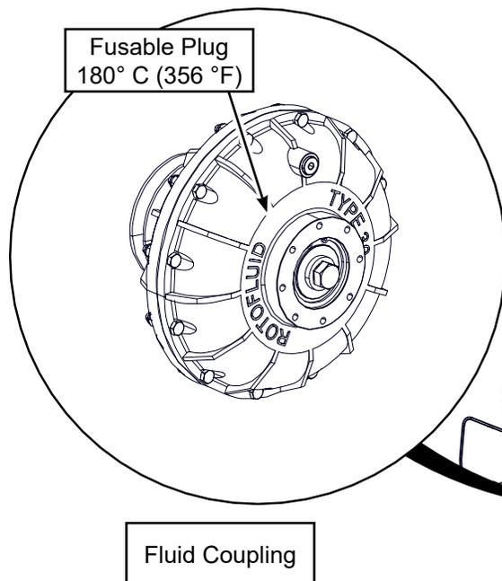
**CAUTION:** Hot Oil and Container: If there is a fluid release from the hydraulic coupler, the oil and container could reach temperatures of 180 °C (356 °F). To prevent severe burns, wait for the oil and container to cool before attempting any maintenance.
