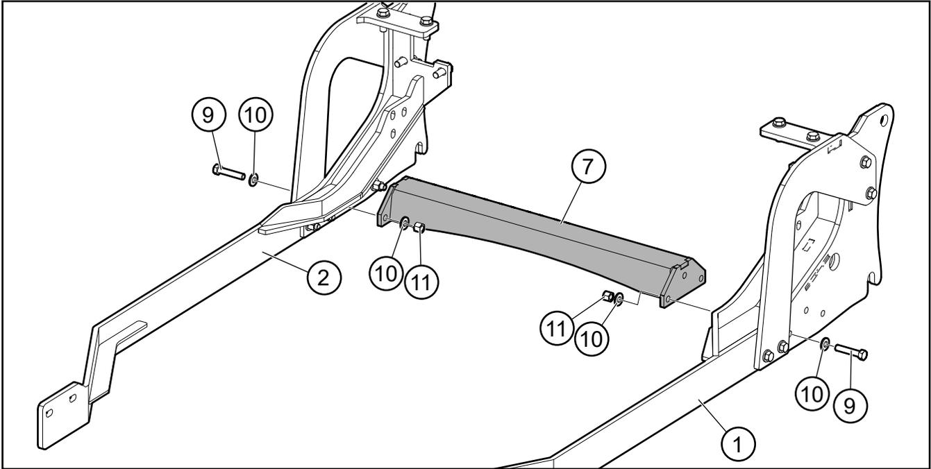
**Torque-tighten all fasteners on the subframe:**
