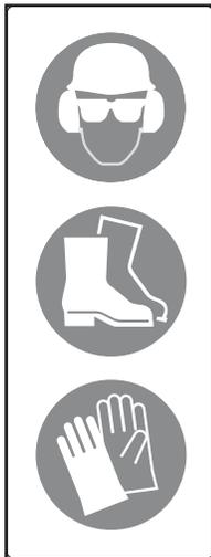
**Information labels** are usually pictorial with a white background and the number of panels can be different. This type gives information to the operator or shows the operation of a control.
