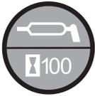
Look for this label on the machine. It indicates a grease point and the interval in hours.
