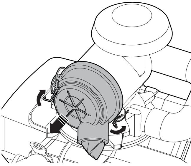
Figure 35—Remove the air-filter cover
