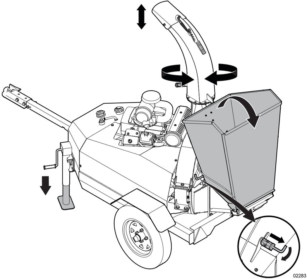
Figure 22 – Set up the machine
