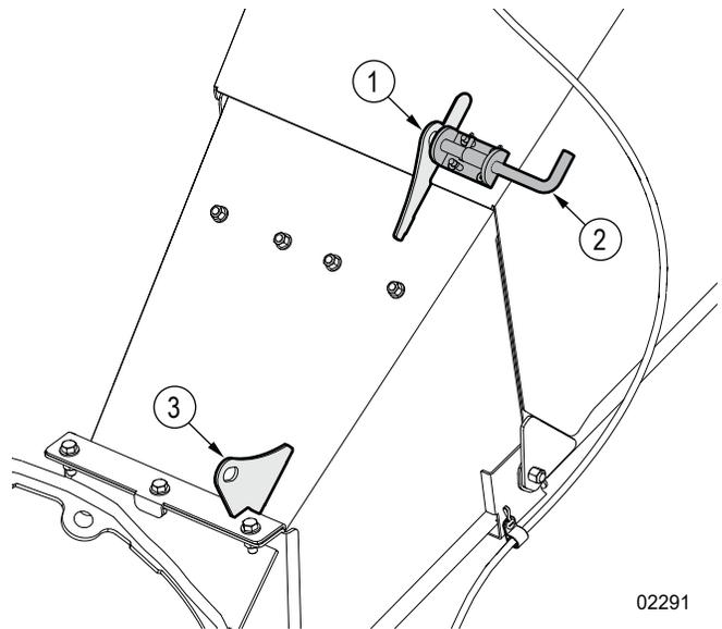
Figure 16—Chipper hopper latch
