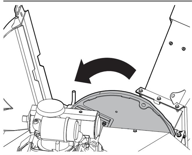
Figure 25—Open the upper rotor housing
