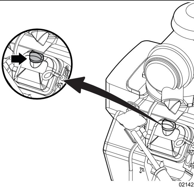
Figure 20—Engine oil-fill location
