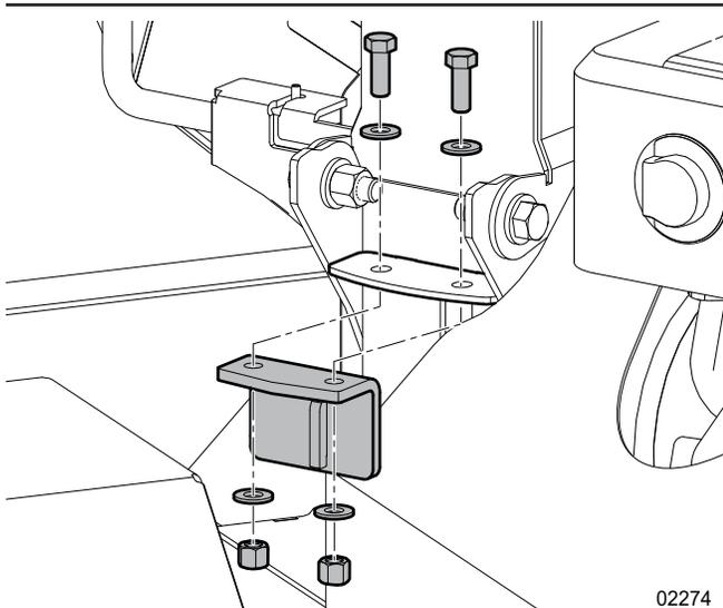
Figure 51 – Install a twig breaker
