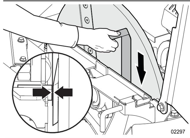
**Figure 50**—Set the ledger knife clearance
