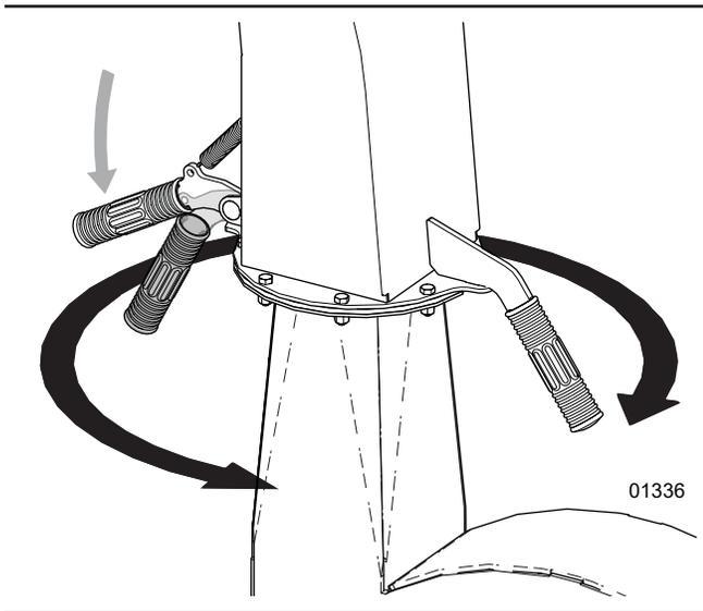
Figure 12—Turn the discharge chute
