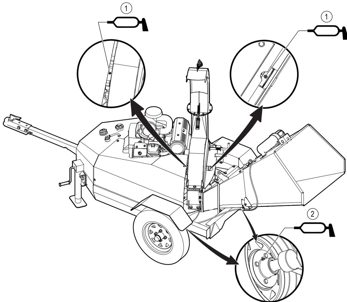
Figure 33—Grease fitting locations
