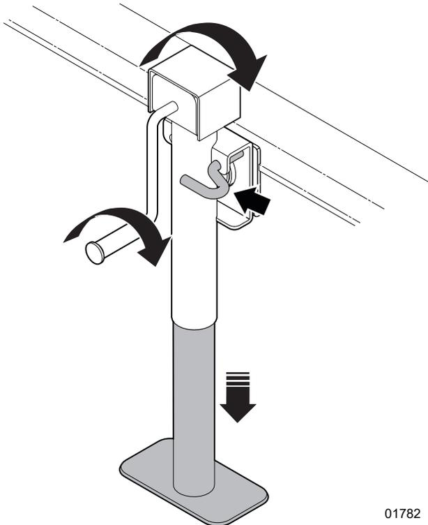
**Figure 30**–Trailer jack in the lowered position
