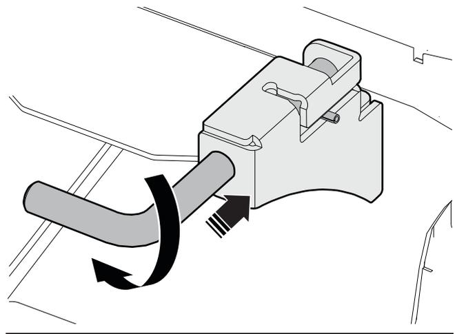
Figure 26—Engage the rotor lock
