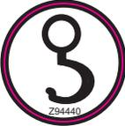
Lifting at this point is the safest way to lift the generator. Have an extra person with a guide rope attached to the generator to prevent swaying.
