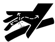
3. Do not attempt any makeshift repairs to the hydraulic lines, fittings or hoses by using tapes, clamps or cements. The hydraulic system operates under extremely high pressure. Such repairs can fail suddenly and create a hazardous and unsafe condition.
