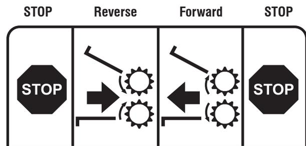
Figure 11—Roller-feed control bar label (right side shown)
