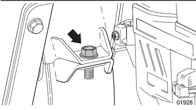
Figure 31 – Upper-rotor-housing retainer bolt
