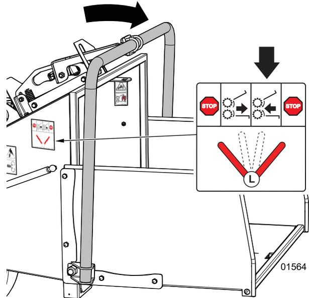
Figure 14—Move material forward (into the machine)
