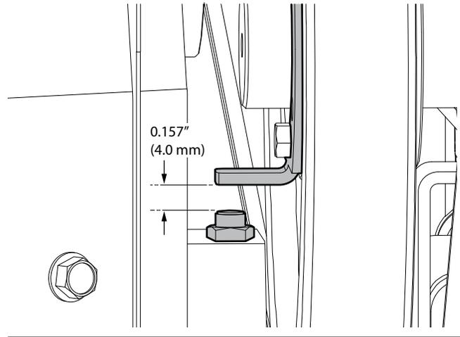
Figure 62—Rotor RPM Sensor position
