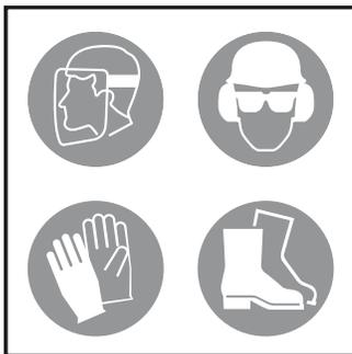
**Information labels** are usually pictorial with a white background and the number of panels can be different. This type of label provides information for the operator or shows the operation of a control.
