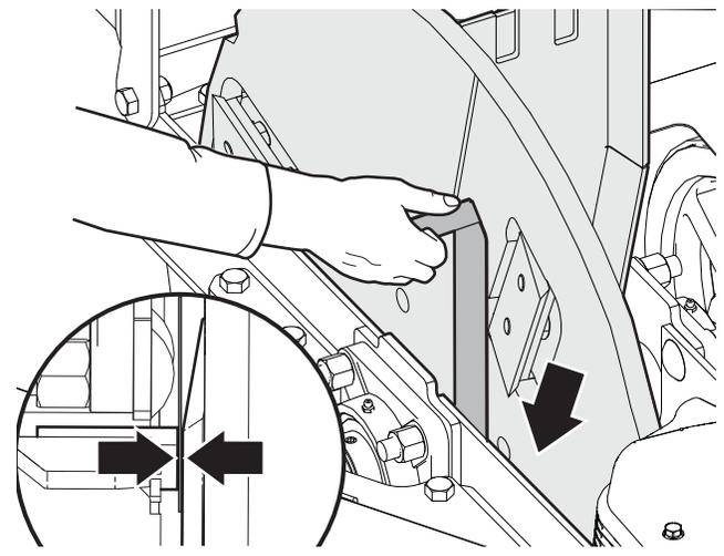
**Figure 60**—Check the ledger knife clearance
