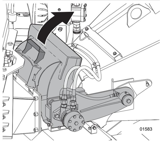
Figure 33 – Roller-feed assembly
