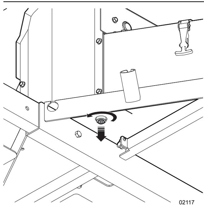
**Figure 44**—Hydraulic-fluid reservoir drain-plug location
