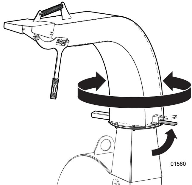
Figure 9 – Turn the discharge chute
