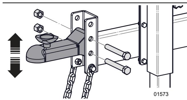
Figure 39—Adjust the hitch-coupler height
