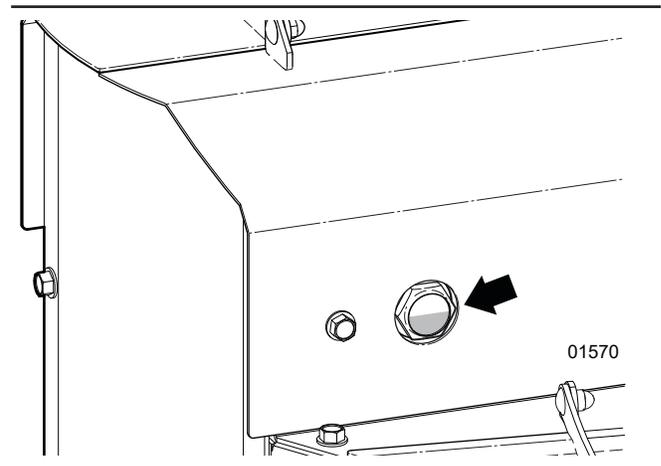
Figure 27 – Hydraulic fluid reservoir fluid level sight glass
