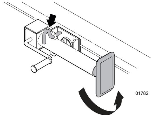
**Figure 38**– Trailer jack in the stowed position
