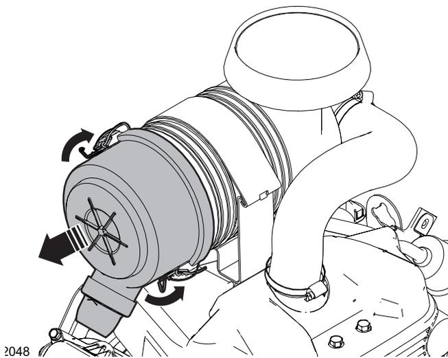
Figure 46—Remove the air-filter cover
