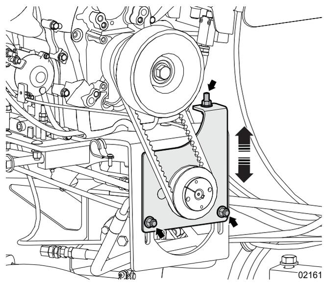
Figure 55—Set the hydraulic pump drive belt tension
