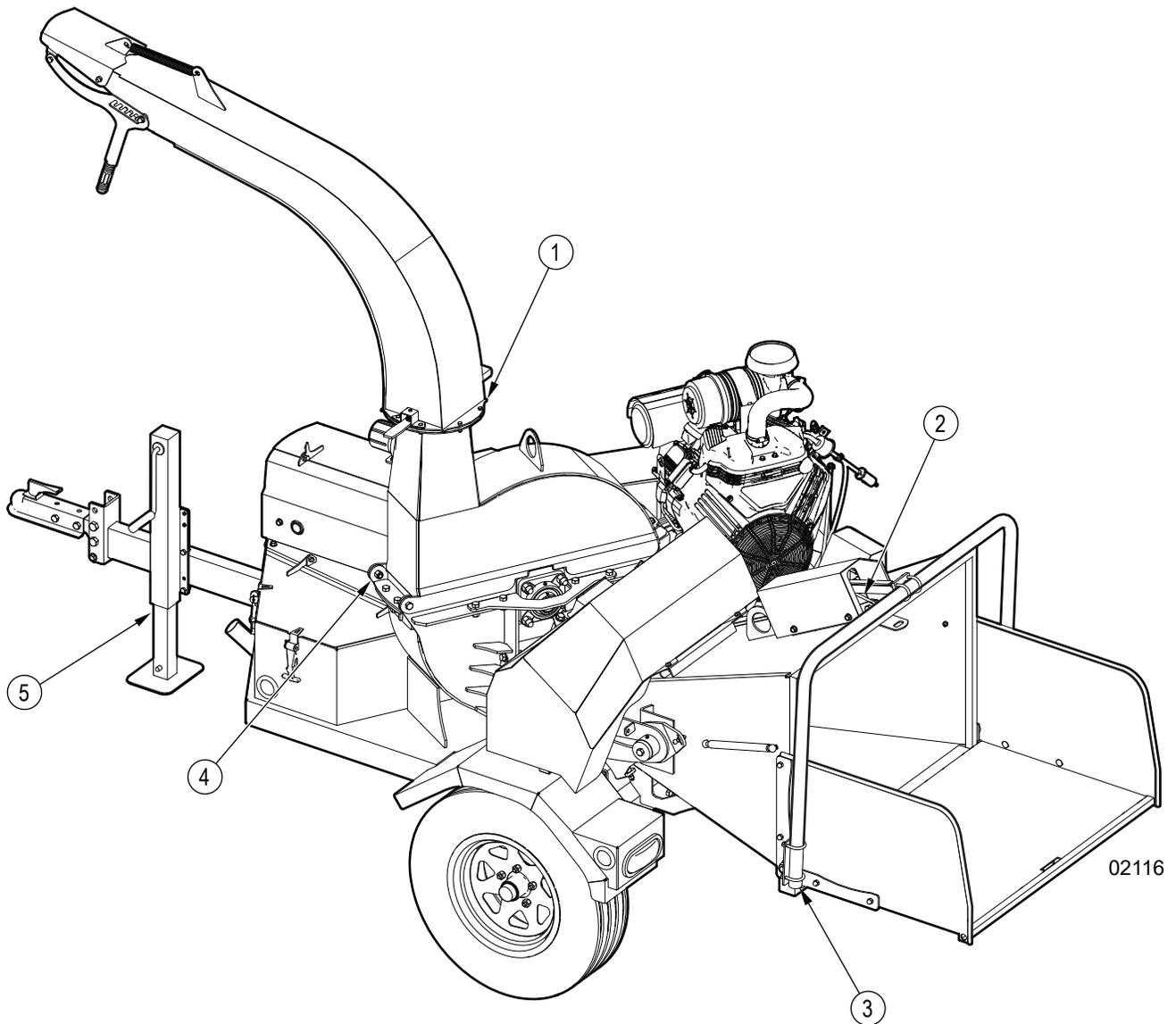
Figure 43—Hinge and pivot point lubrication locations
