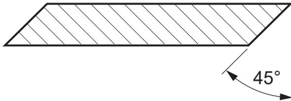
**Figure 57**—Sharpen rotor knives to a 45° angle
