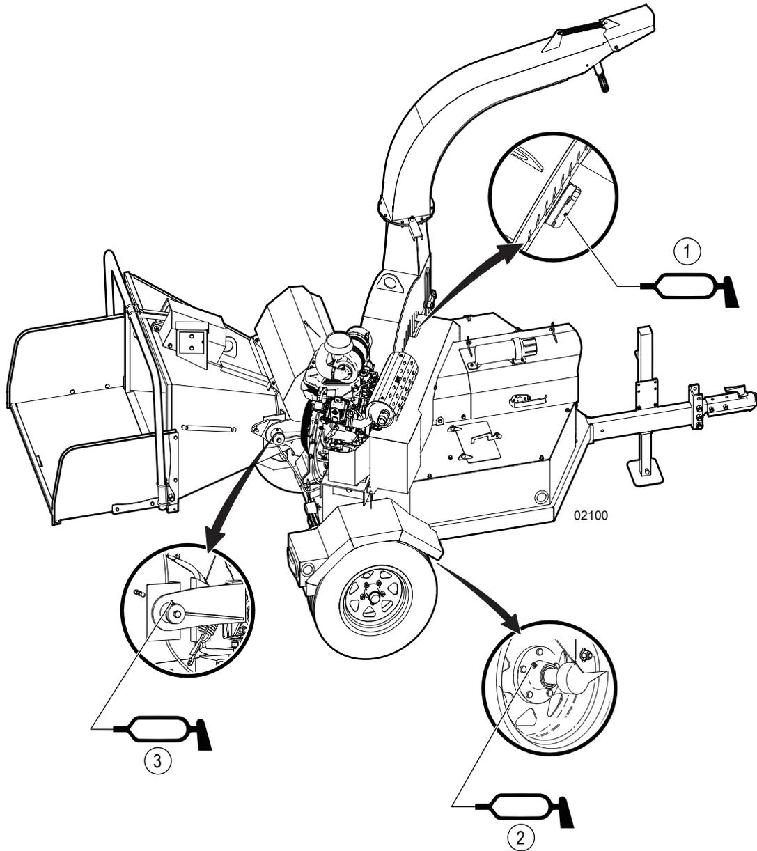
Figure 41 – Grease fitting locations - right side
