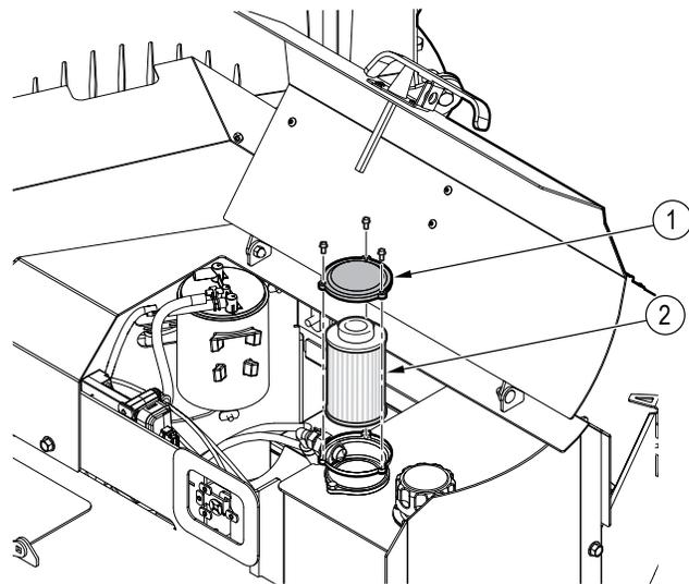
**Figure 45**—Hydraulic fluid filter
