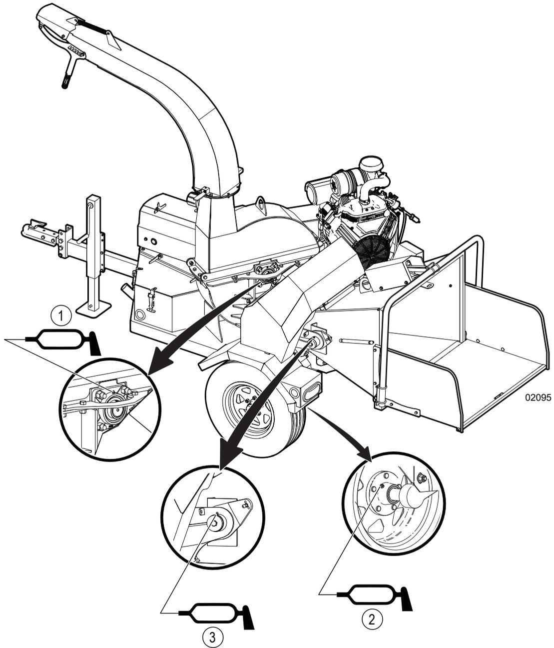
Figure 42—Grease fitting locations - left side
