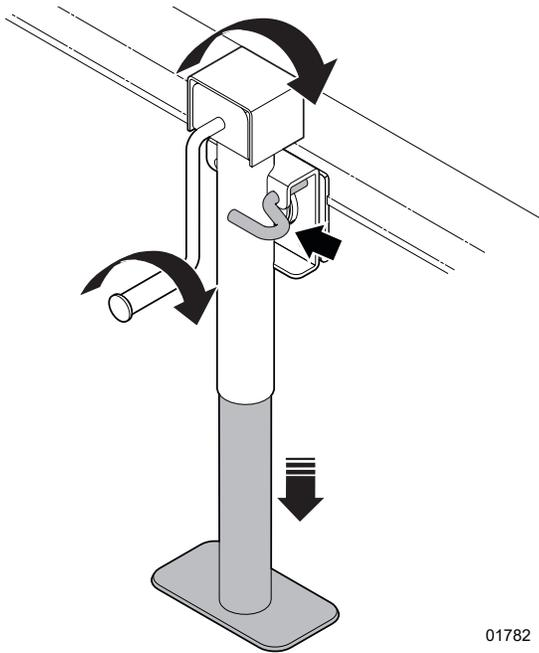
**Figure 37**– Trailer jack in the lowered position
