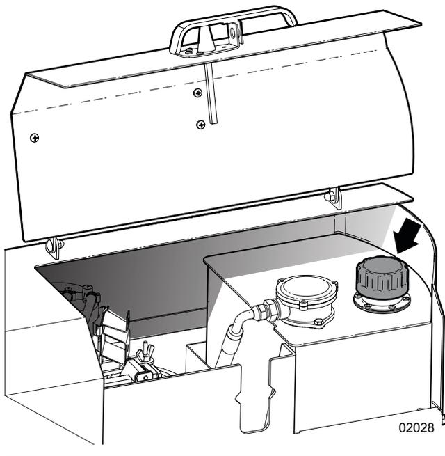
Figure 28—Hydraulic fluid reservoir fill cap
