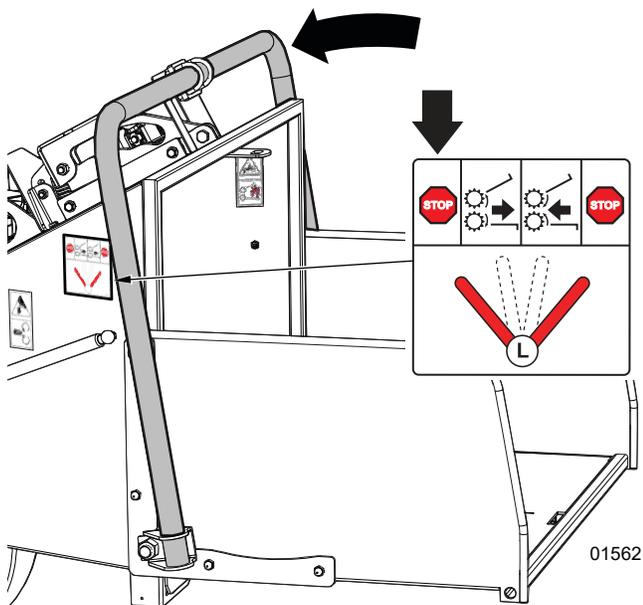
Figure 12—Forward STOP position
