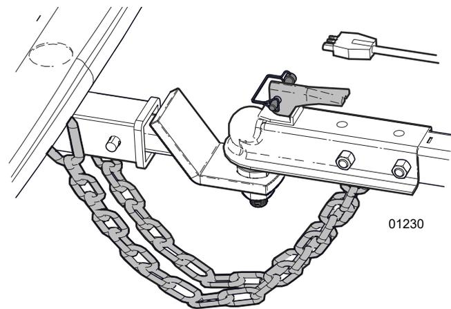
Figure 36—Ball-mount hitch connection
