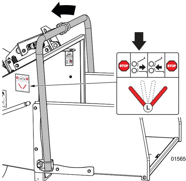
Figure 15—Move material to the rear (out of the machine)
