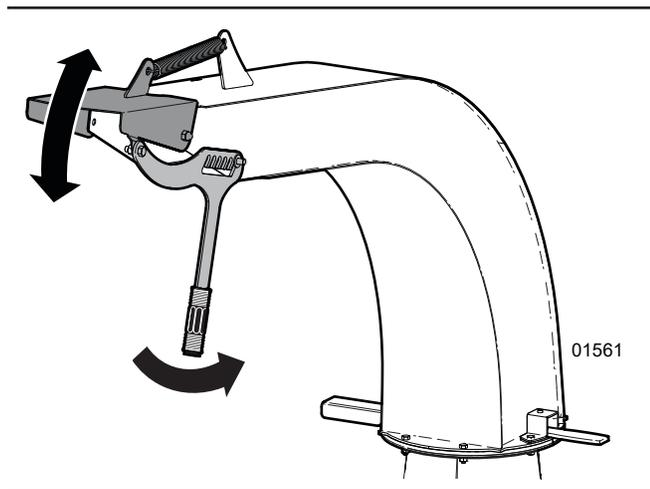
Figure 10—Adjust the hood deflector
