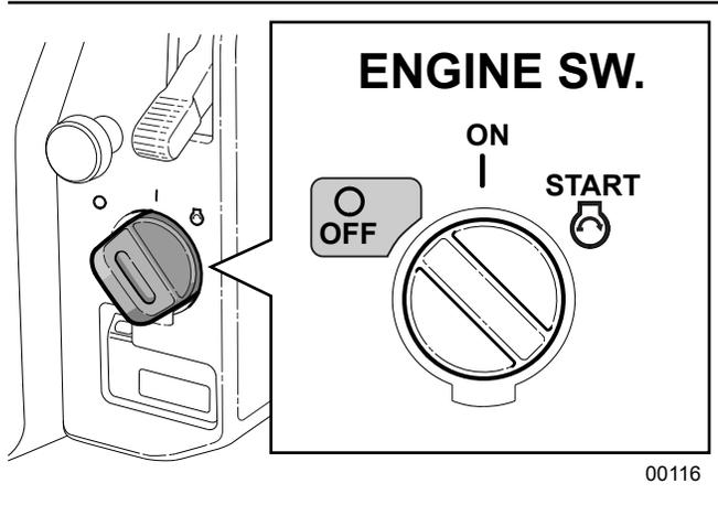
Fig. 9—Engine Start Switch
