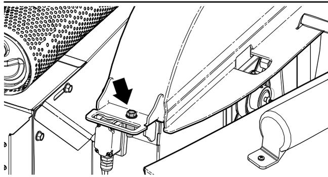
Fig. 42 – Rotor Housing Flange Bolt
