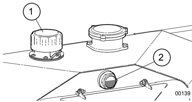
**Fig. 33**—Hydraulic Tank Oil Level Check
