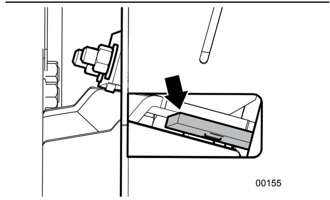
Fig. 72—View of Ledger Knife from underside of Chipper
