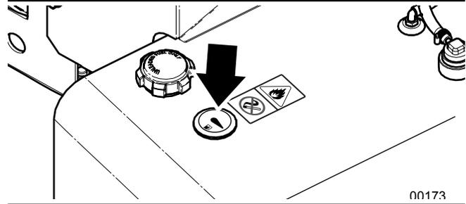
Fig. 30—Fuel Level Gauge
