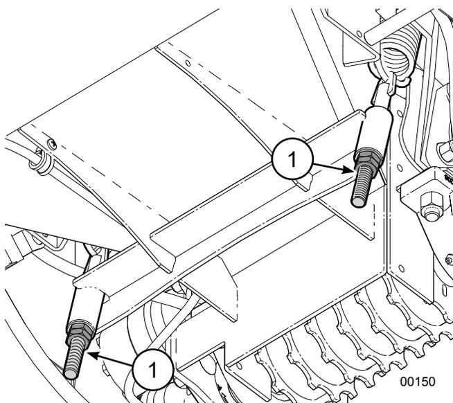
Fig. 66—Upper feed roller tensioner (US model shown)
