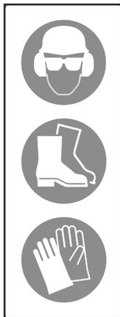
**Information labels** are usually pictorial with a white background and the number of panels can be different. This type of label provides information for the operator or shows the operation of a control.
