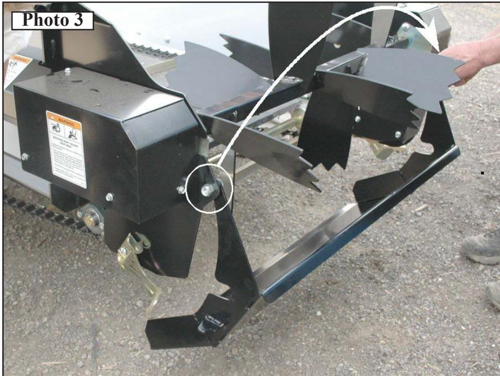
4. Swing Fines Pan down to brackets and secure with Lynch Pin. *Photo 4*
