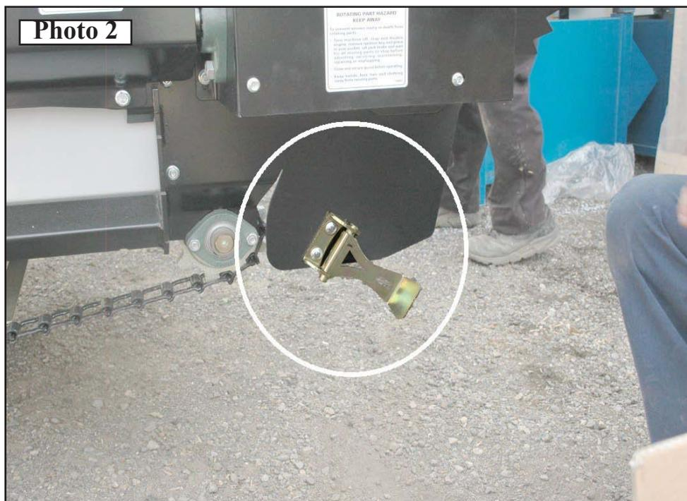
3. Attach the Fines Pan at the brackets on rear of spreader and secure with (2) **Hex Bolt 1/2NC** & (2) **Hex Locknut 1/2NC**. *Photo 3*
