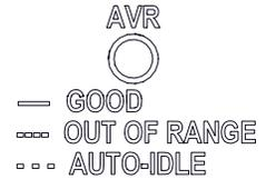
**Auto Idle:** When there is no load detected, the AVR indicator light will blink slowly, and the engine will slow to an idle. This feature is switchable on or off.
