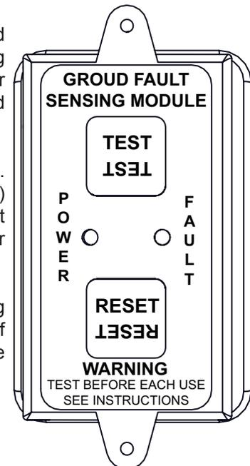
Note: An electrical overload is indicated if the breaker trips and the GFCI green power light is still on.
