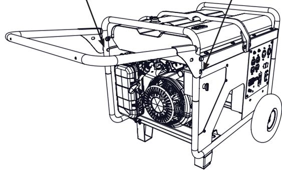
Do not lift entire generator by folding handle. Folding handle is not intended for motorized transport of generator.
