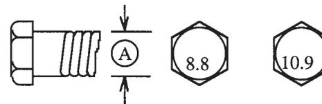
Torque figures indicated above are valid for non-greased or non-oiled threads and heads unless otherwise specified. Therefore, do not grease or oil bolts or capscrews unless otherwise specified in this manual. When using locking elements, increase torque values by 5%.
