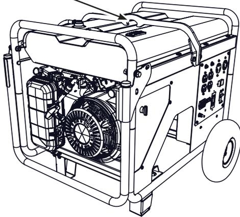
person with a guide rope attached to the generator to prevent swaying.
