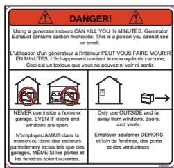
**Danger:** Never run a generator indoors, a generator's exhaust contains toxic carbon monoxide, which you cannot smell or see. Breathing carbon monoxide can be lethal.
