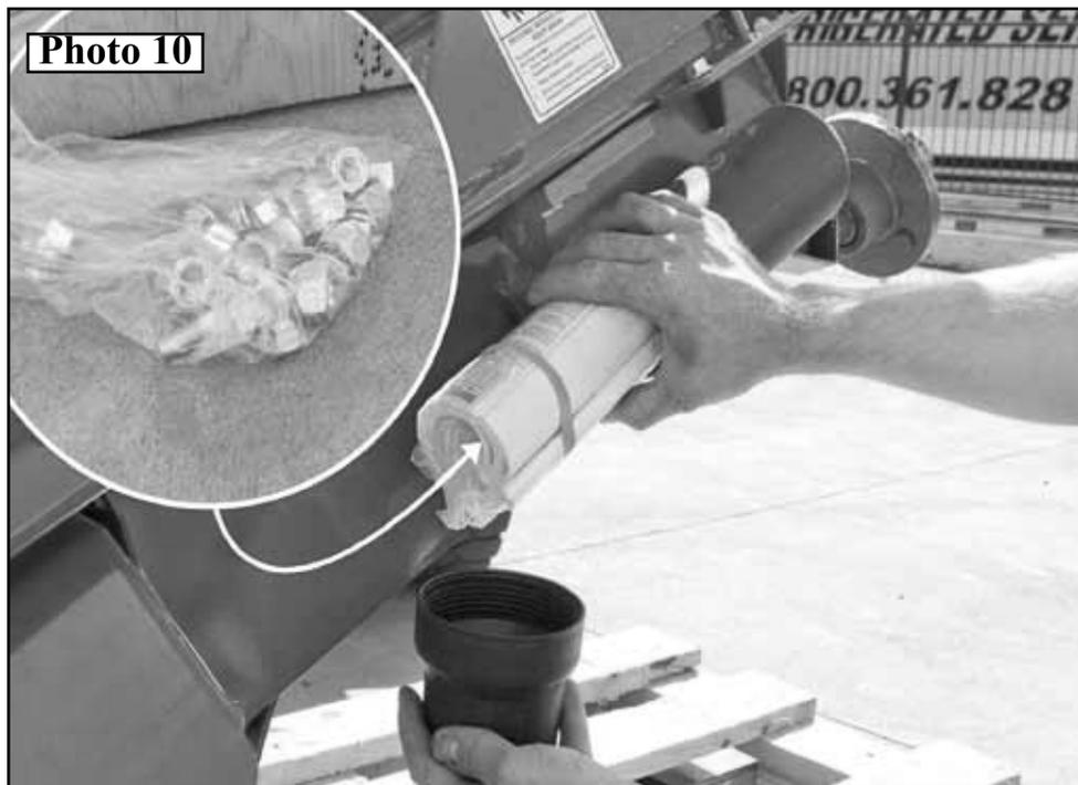
10. Secure the 2" Hitch Coupler at the Splitter using four 1/2" Locknut *Photo 11*
