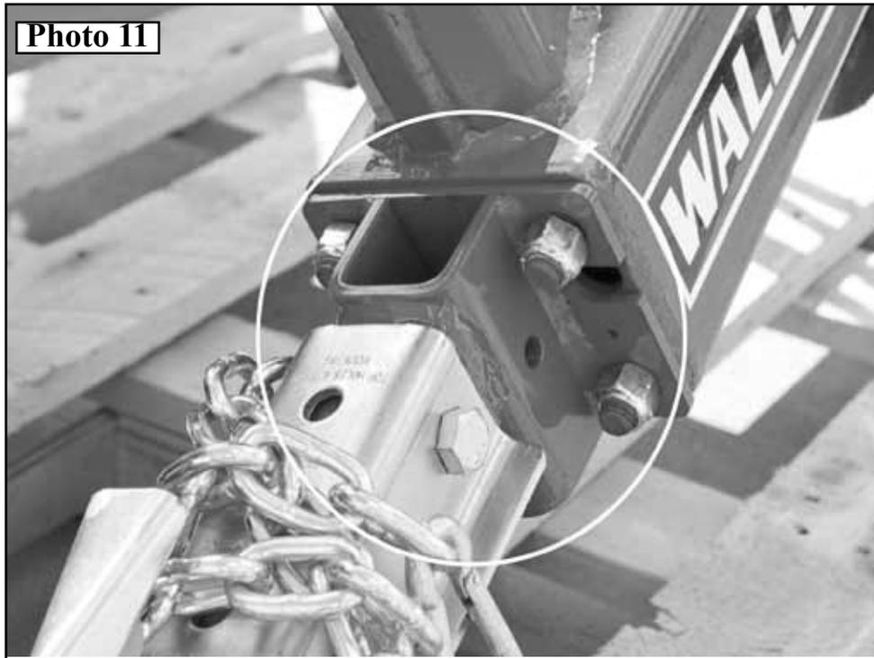
11. Slide Front Jack into position at 2" Hitch Coupler Assy and secure with one (1) Snapper Pin 3/8 x 2-1/4 *Photo 12*
