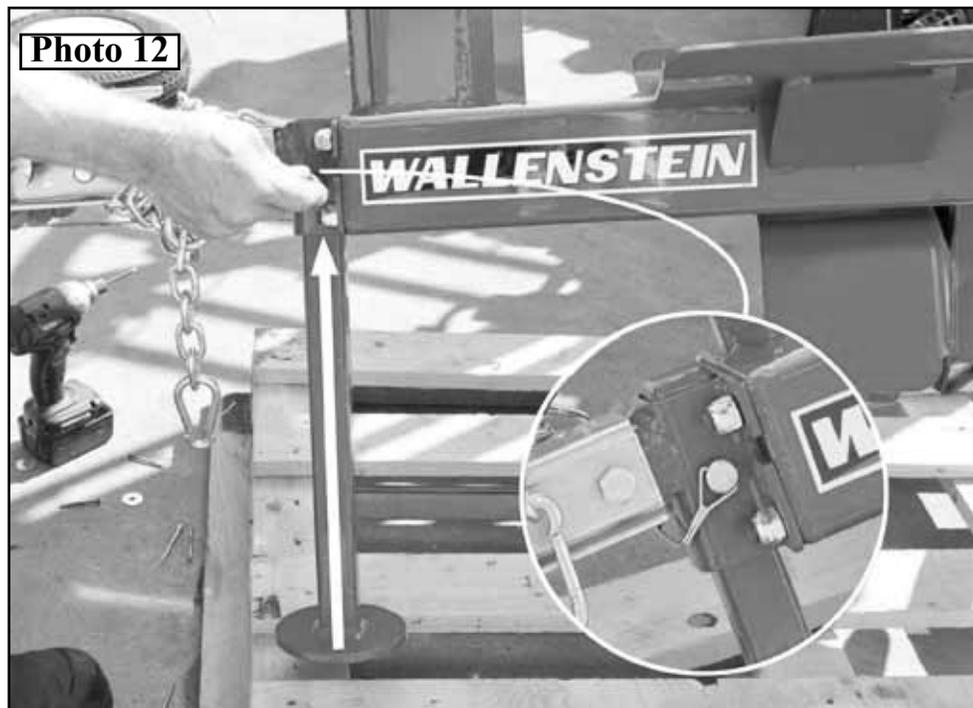
12. Swivel Axle Assembly 90 degrees to Main Base Weldment. *Photo 13*
