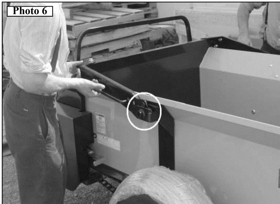
6. Insert End Gate Pivot Pin, aligning the hole of pin with hole in welded bushing on End Gate Pivot Base. *Photo 7*
