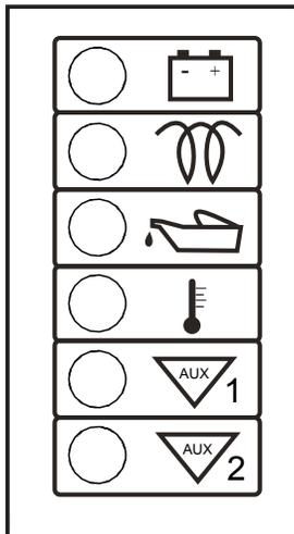
**Battery:** lights up when the ignition is set to "run", the indicator shuts off after the engine starts.
