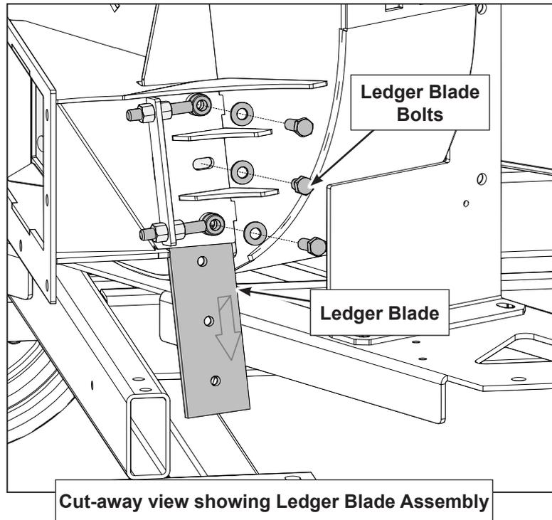
**For fast and easy setting, use the chipper clearance setting gauge, included with the machine. Replacements available from your dealer (see accessories).**
