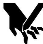
**Risk of pinching or crushing hazard! Never reach into the splitting cradle to reposition a log. Use a log peavy (cant hook) or other tool.**
