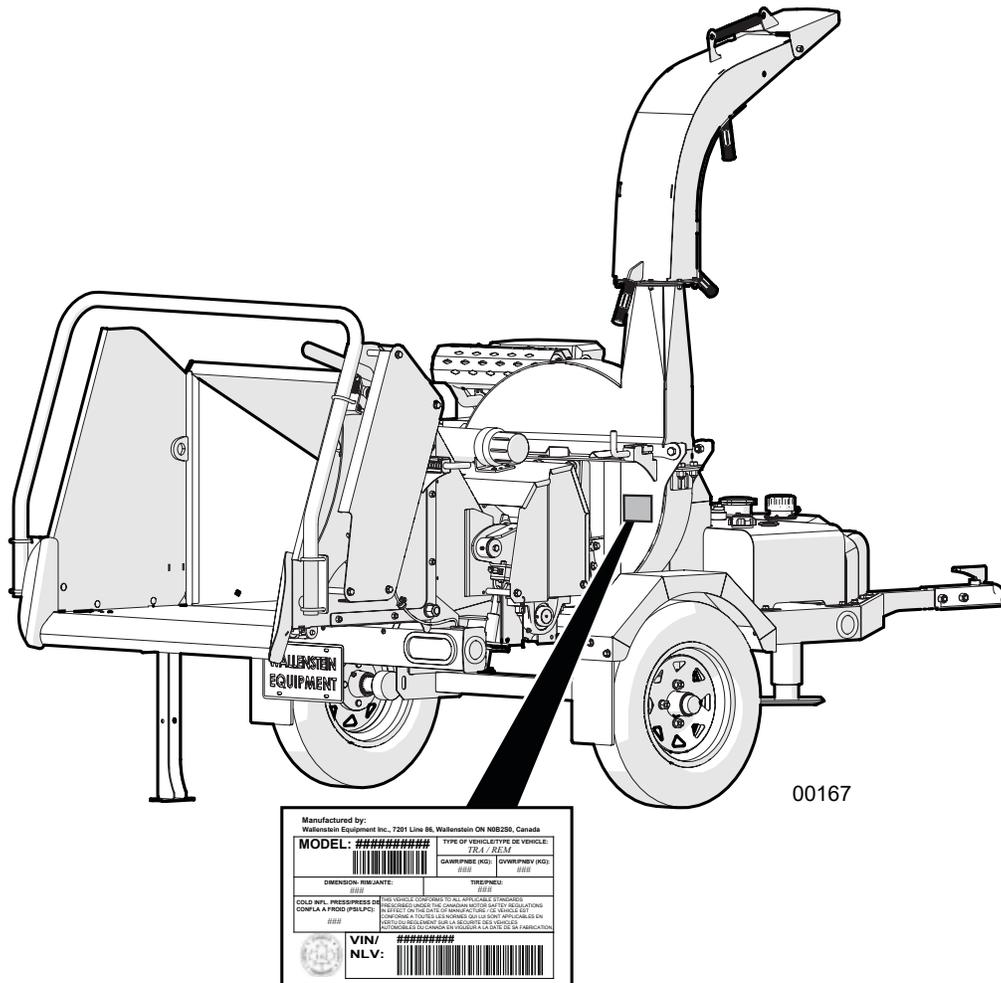
Fig. 1 – Serial Number Plate Location
