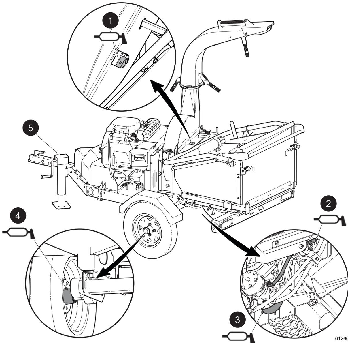
Fig. 49–Grease Points – 50 Hours of Operation or Annually
