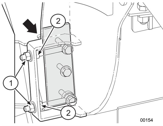
Fig. 69—Adjusting ledger knife clearance
