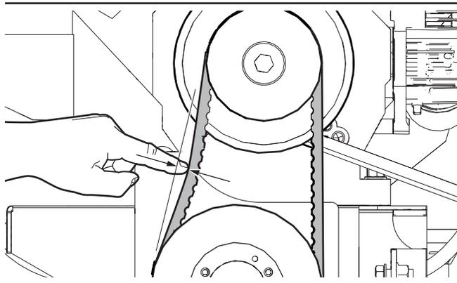
Fig. 60—Drive belt tension
