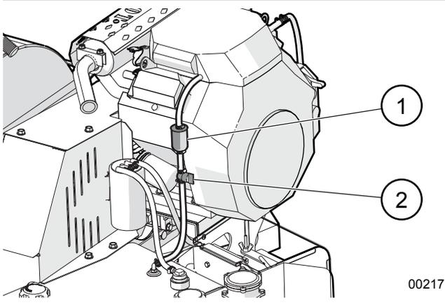
Fig. 73—Engine Fuel Filter
