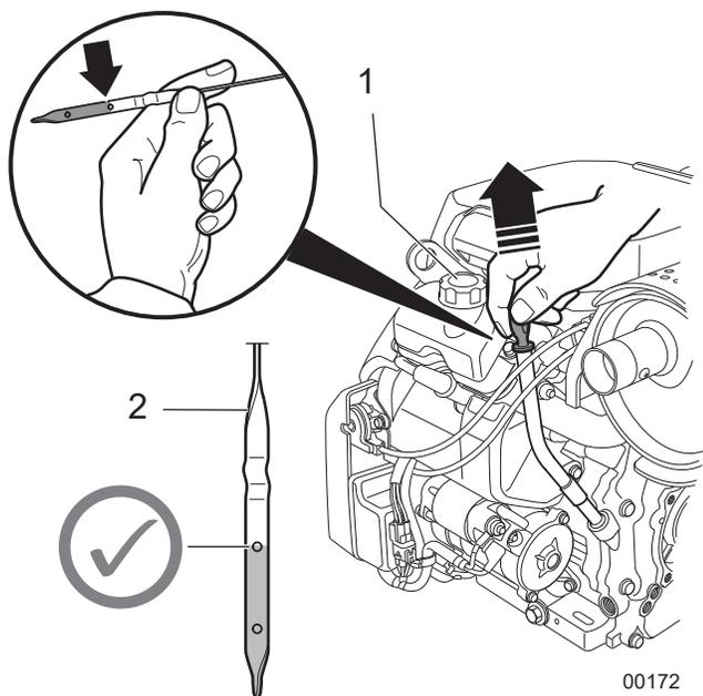
**Fig. 31**—Checking Engine Oil Level
