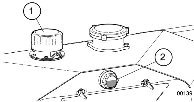
**Fig. 32**—Hydraulic Tank Fluid Level Check
