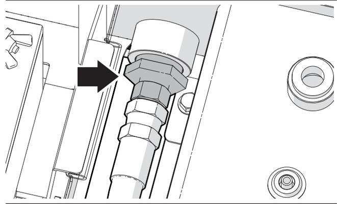
Fig. 53 – Suction Strainer on Hydraulic Tank
