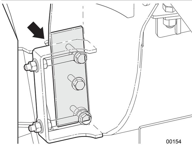
Fig. 67—Ledger knife inside lower rotor housing
