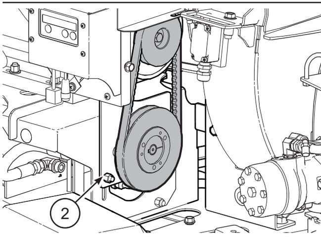
Fig. 58—Bolts holding pump mounting plate
