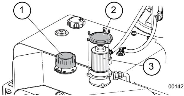
**Fig. 55**—Hydraulic Fluid Filter Element
