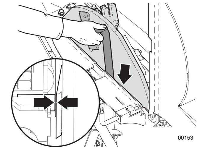
Fig. 68—Checking ledger knife clearance
