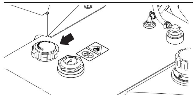
Fig. 30 – Fuel tank Cap
