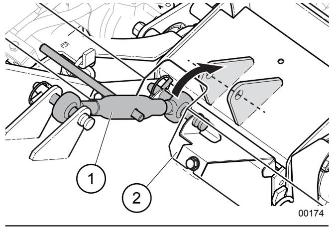
Fig. 43 – Connect Toplink to Bridge
