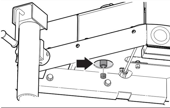
Fig. 52 – Hydraulic Tank Drain Plug
