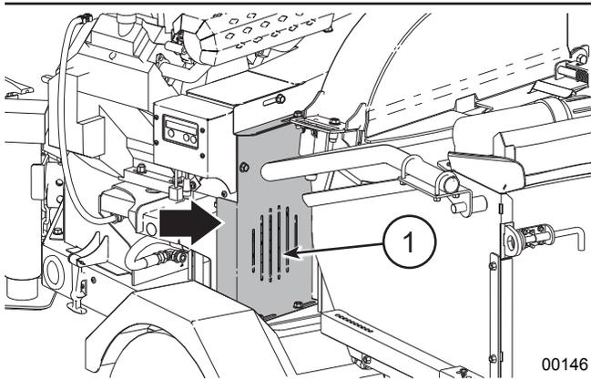
Fig. 57—Lower drive belt shield
