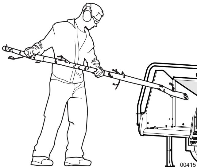
Fig. 40—Stand to Side of Feed Table
