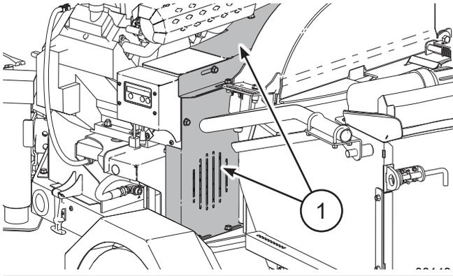
Fig. 61—Upper and lower drive belt shields
