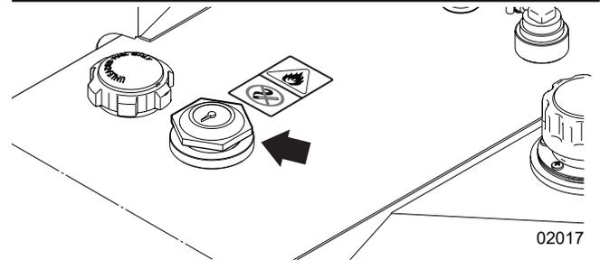
Fig. 29 – Fuel Level Gauge
