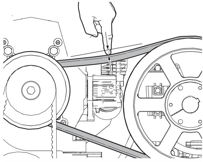
Fig. 64—Rotor drive belt tension
