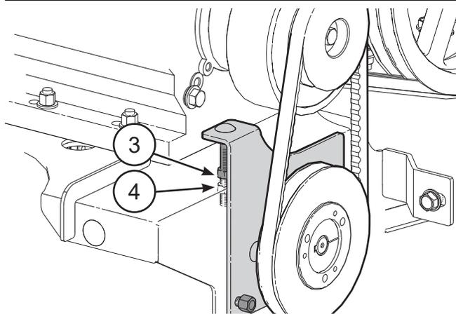
Fig. 59—Belt Tension Adjuster
