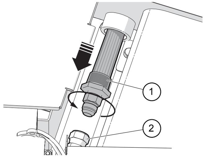
Fig. 54 – Suction Strainer on back of Hydraulic Tank
