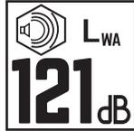
Always wear hearing protection when near the operating machine. Noise exposure over 85 dB on a long-term basis can cause severe hearing loss. Exposure over 90 dB over a long-term basis may cause permanent, total hearing loss.
