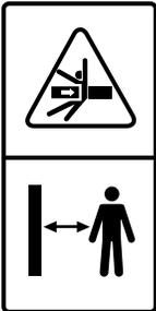
Risk of collision / crushing / pinching injury from the grapple forks when it rotates.
