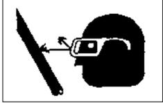
3. Do not attempt any makeshift repairs to the hydraulic lines, fittings or hoses by using tapes, clamps or cements. The hydraulic system operates under extremely high pressure. Such repairs will fail suddenly and create a hazardous and unsafe Condition.
