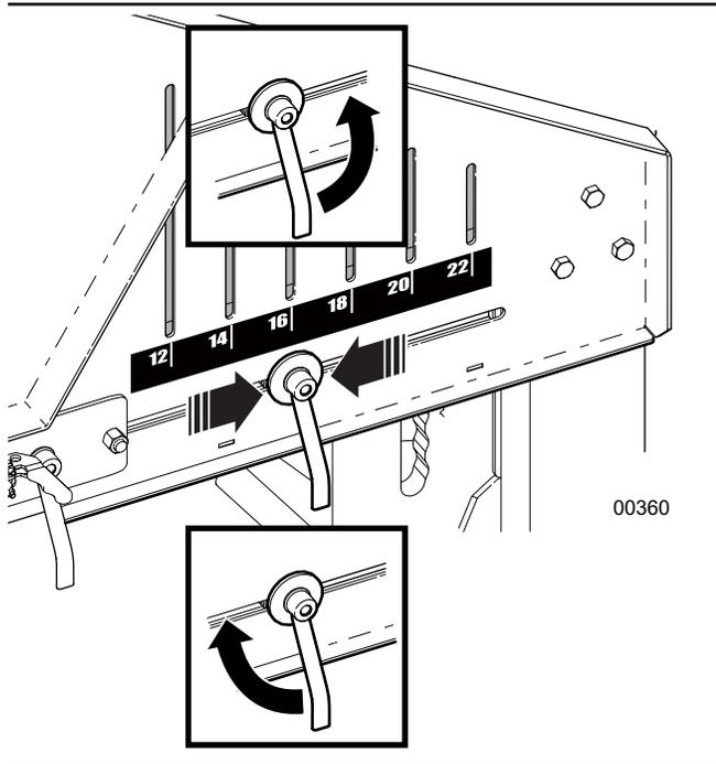
Fig. 29—Log Stop Guide Lock Handle
