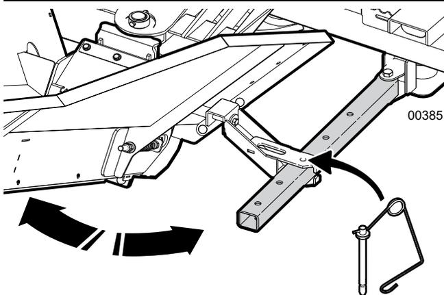
Fig. 36—Set the Conveyor Angle
