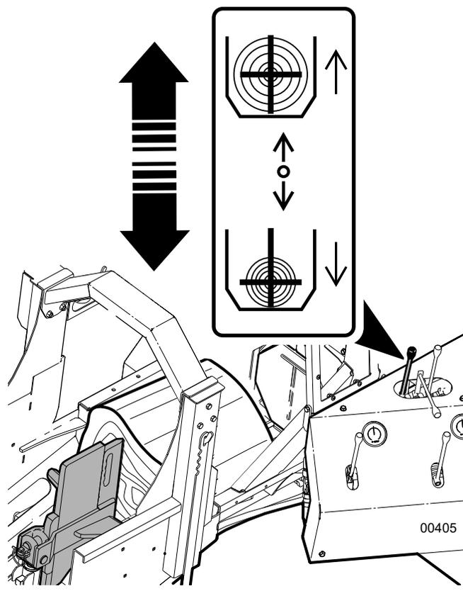
Fig. 61—Adjust Wedge Height
