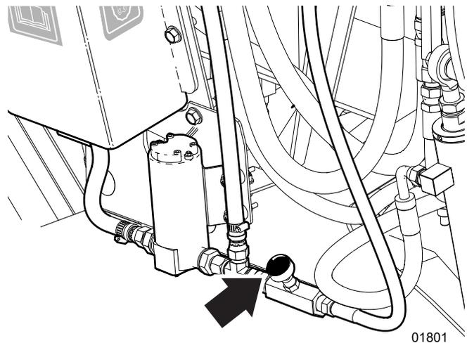
Fig. 60 – Bar Oil Flow Control
