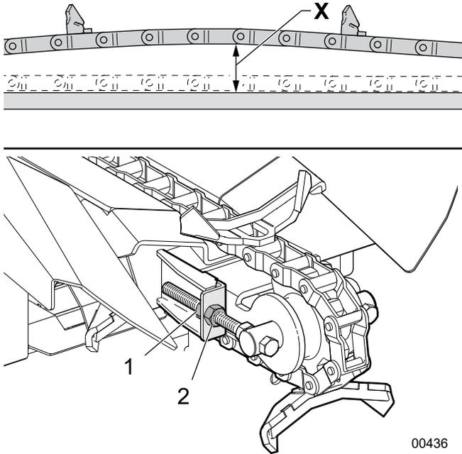
**Fig. 91** – Infeed Conveyor Chain
