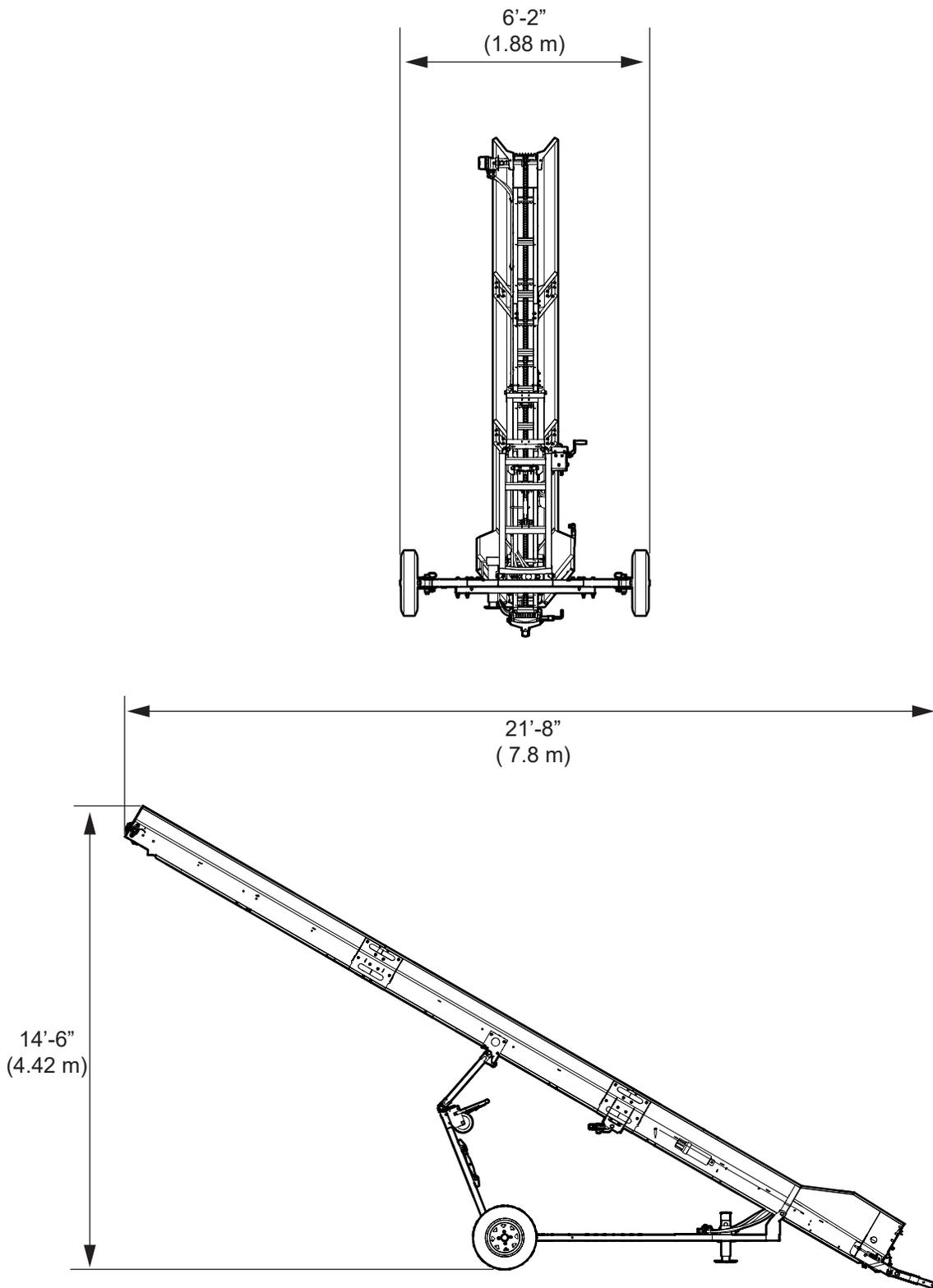
Fig. 103–24 ft Conveyor Dimensions
