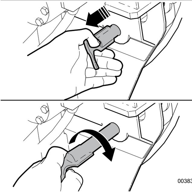
Fig. 23—Live Deck Locking Pins
