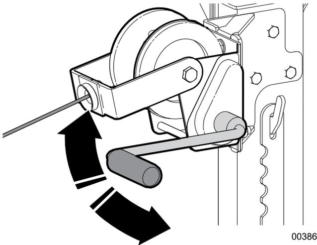
Fig. 35—Conveyor Hand Winch
