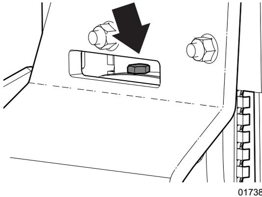
**Fig. 88**—Adjusting Screw
