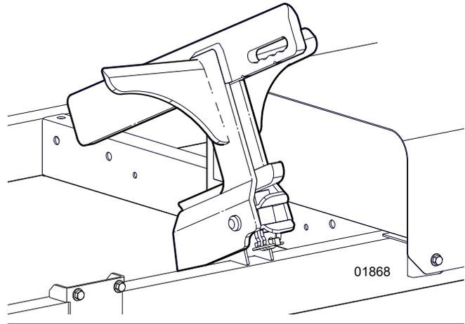
Fig. 65—Splitting Wedge Storage
