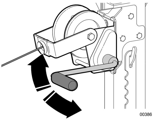
Fig. 14—Conveyor Hand Winch
