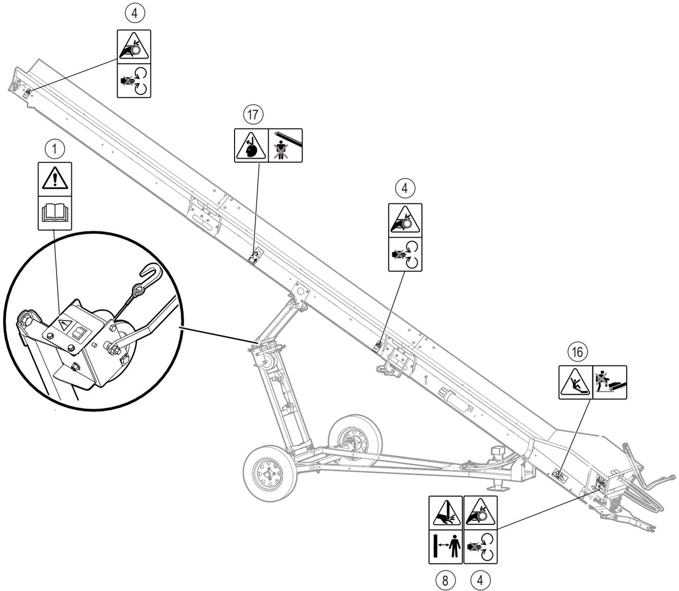
Fig. 7- 24 ft Conveyor Safety Decal Locations
