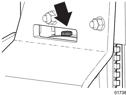
Fig. 58 – Adjusting Screw
