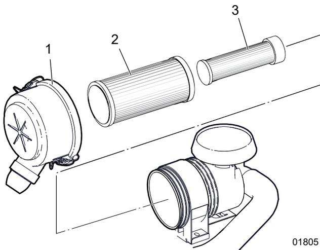
Fig. 83—Cyclonic Engine Air Cleaner
