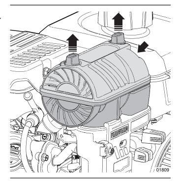
Figure 33 - Engine air filter
