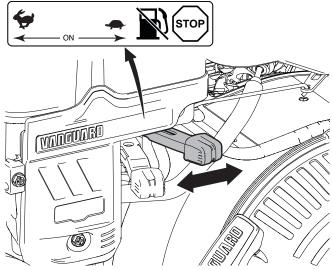
Figure 9-Engine throttle control and fuel shutoff
