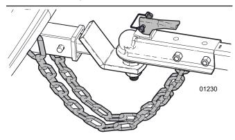
Figure 27 - Ball-mount hitch connection
