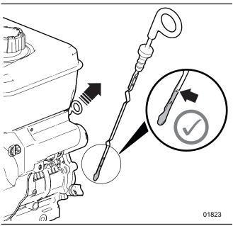
Figure 18-Check the engine oil level
