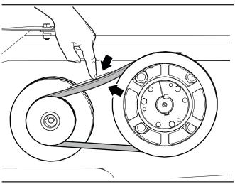
Figure 37 - Check the drive belt tension
