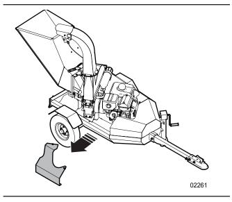
Figure 34-Remove the engine guard
