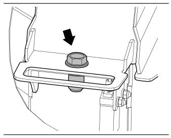
Figure 22 - Upper-rotor-housing fastener
