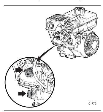
Figure 19 - Engine oil-fill locations
