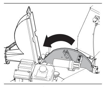
Figure 23-Open the upper rotor housing
