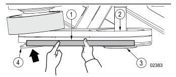
Figure 41 – Align the engine clutch
