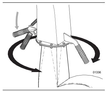
Figure 13 - Turn the discharge chute
