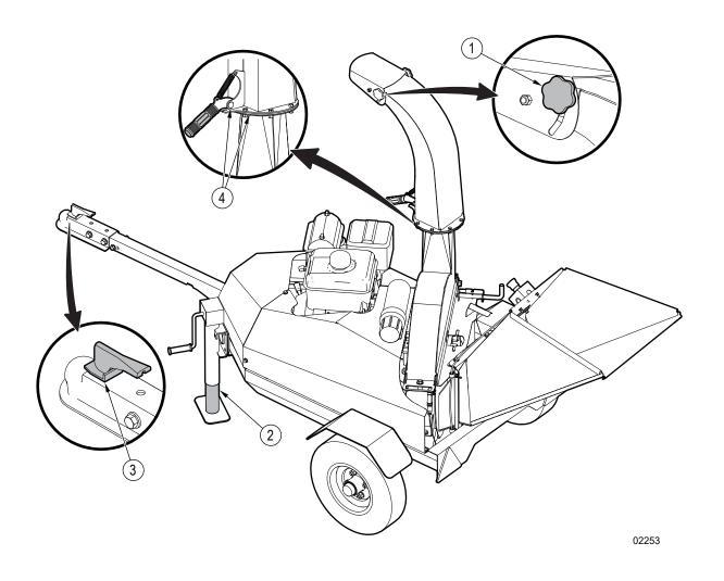
Figure 32 – Hinge and pivot point grease locations
