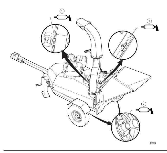
Figure 31 – Grease fitting locations
