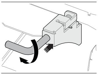
Figure 24 - Engage the rotor lock
