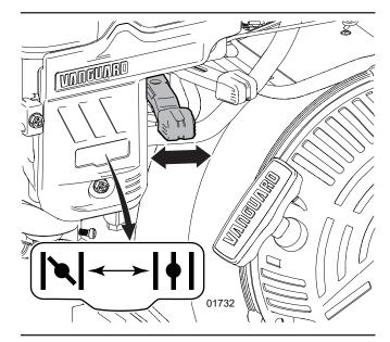
Figure 10 - Engine choke control
