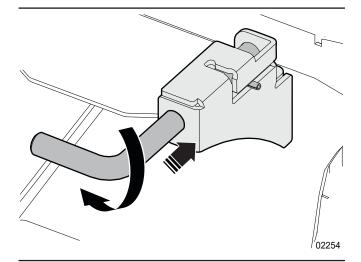
Figure 15-Engaged position
