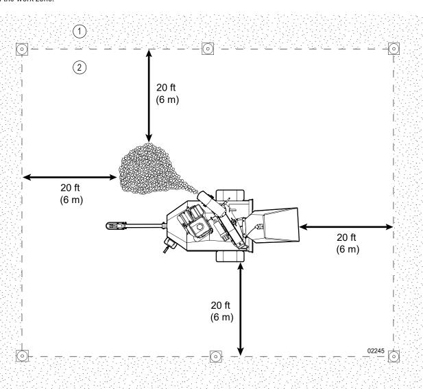
Figure 2-Example of a safe work area
