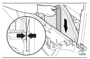
Figure 48 - Set the ledger knife clearance
