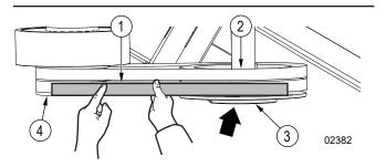
Figure 42 - Align the rotor sheave
