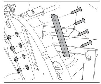
Figure 44-Install a rotor knife
