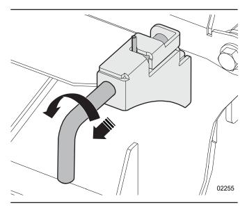
Figure 25 - Disengage the rotor lock
