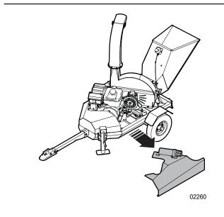
Figure 35 - Remove the drive-belt guard
