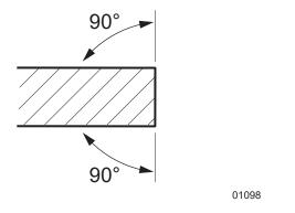
Figure 47 - Sharpen a ledger knife
