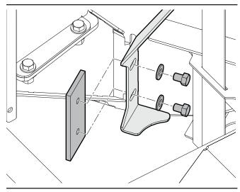
Figure 46-Install a ledger knife
