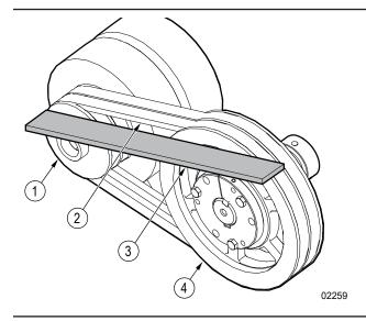
Figure 40 - Check the drive belt alignment
