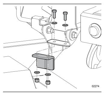
Figure 49-Install a twig breaker
