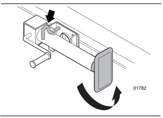
Figure 29 - Trailer jack in the stowed position
