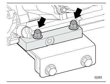
Figure 39 – Engine mount bolts (two of four)
