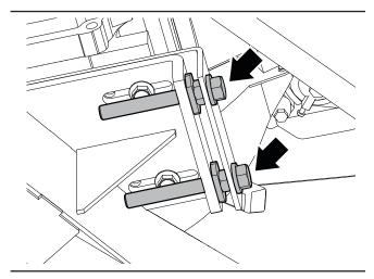
Figure 38 - Drive belt tensioning bolts
