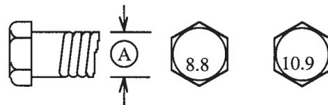
Torque figures indicated above are valid for non-greased or non-oiled threads and heads unless otherwise specified. Therefore, do not grease or oil bolts or capscrews unless otherwise specified in this manual. When using locking elements, increase torque values by 5%.
