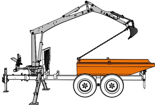
**⚠ Caution:** Ensure pivot tubes snap lock pins are in place to secure the dump box to the trailer.
