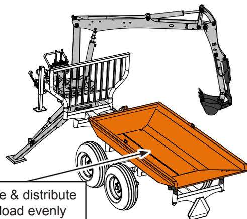
**⚠ Caution:** Ensure pivot tubes snap lock pins are in place to secure the dump box to the trailer.
