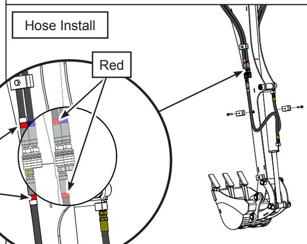
Cutaway view showing hydraulic connections.
