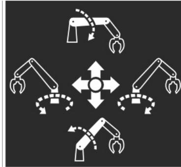
3. **Dipper Boom: Up / Down & Bucket In / Out**
