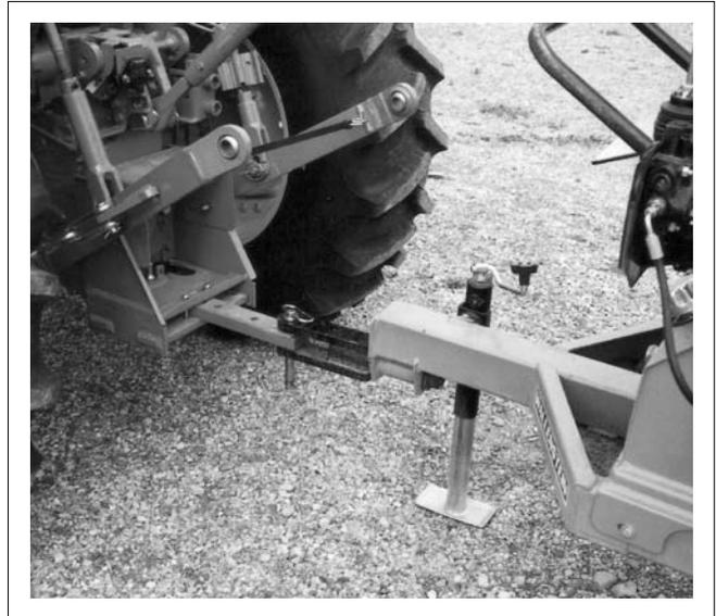
**Fig. 4 DRAWBAR PIN AND RETAINER**
