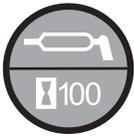
Look for this decal on your machine. It indicates a grease point and the interval in hours.
