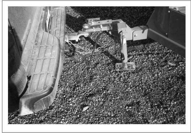
**Fig. 16 STAND/WIRING HARNESS**
