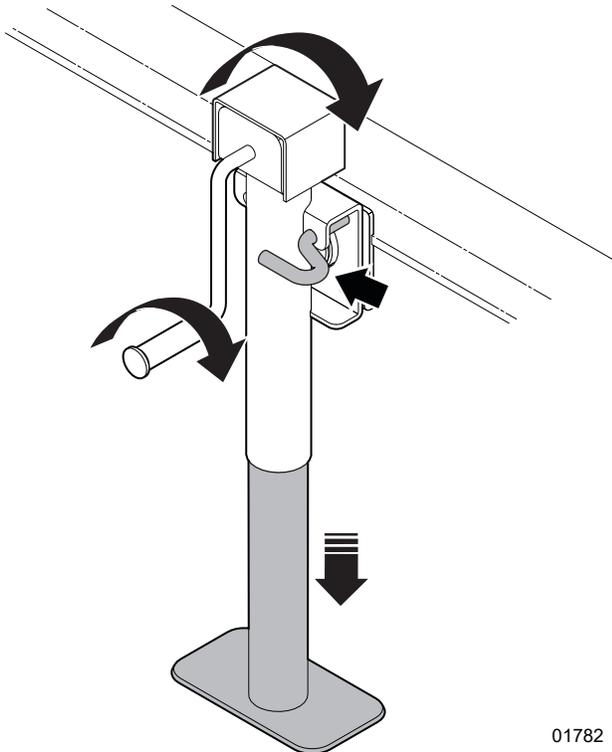
**Figure 28**–Trailer jack in the lowered position
