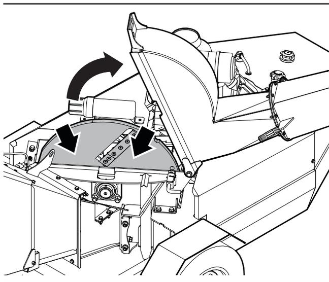
Figure 23—Open the upper rotor housing
