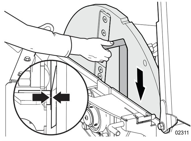
**Figure 48**—Set the ledger knife clearance
