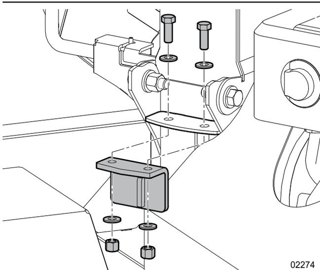
Figure 49—Install a twig breaker
