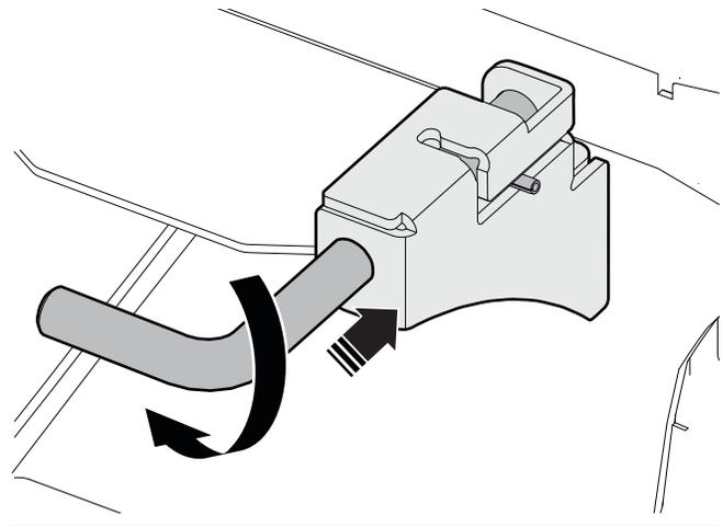
Figure 24—Engage the rotor lock
