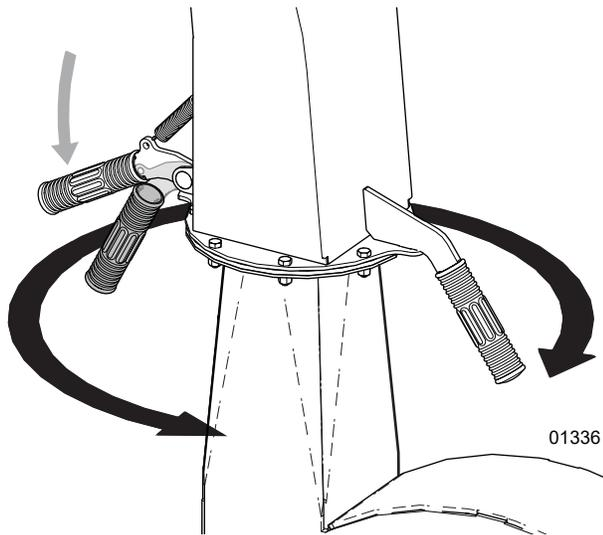
Figure 10 – Turn the discharge chute
