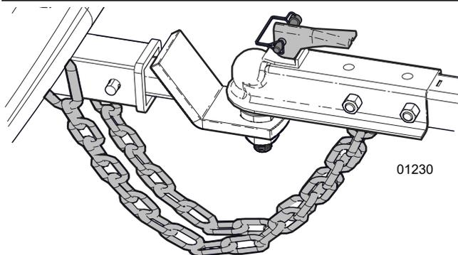
**Figure 27**—Ball-mount hitch connection
