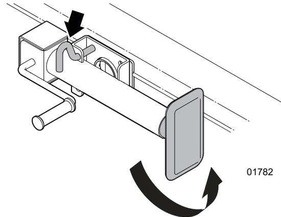
**Figure 29**–Trailer jack in the stowed position
