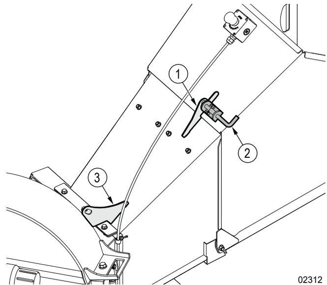
Figure 14—Chipper hopper latch
