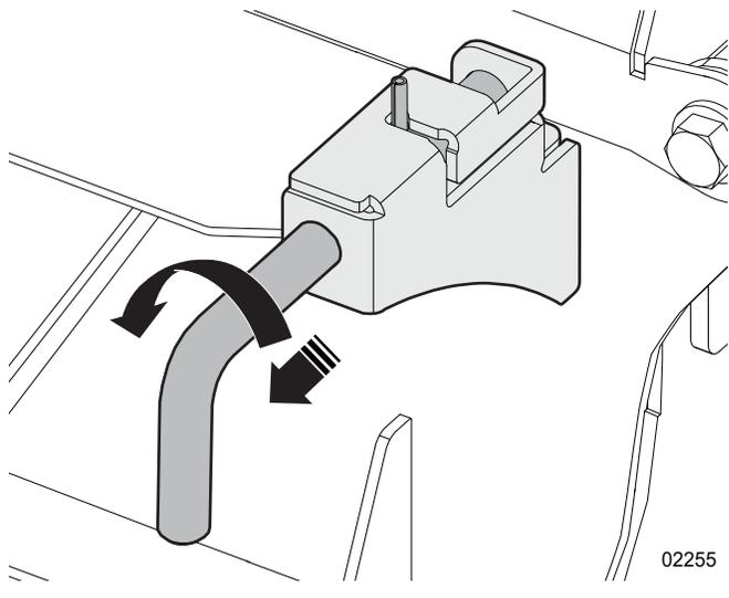
Figure 25—Disengage the rotor lock
