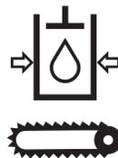
This gauge indicates the saw circuit operating pressure.
