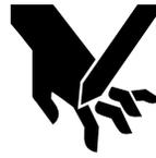
Risk of pinching or crushing hazard! Never reach into the splitting cradle to reposition a log. Use a log peavey, hookaroon or another tool.
