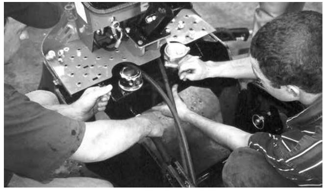
Fig. 5—Installing Reservoir in Backhoe Frame
