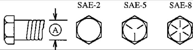
Torque figures indicated above are valid for non-greased or non-oiled threads and heads unless otherwise specified. Therefore, do not grease or oil bolts or capscrews unless otherwise specified in this manual. When using locking elements, increase torque values by 5%.
