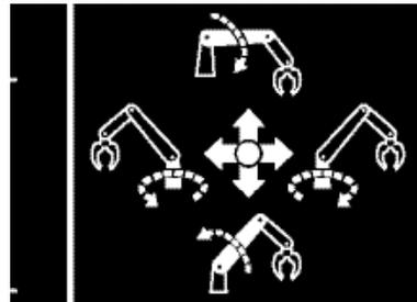
3. **Dipper Boom: Up / Down & Bucket In / Out**
