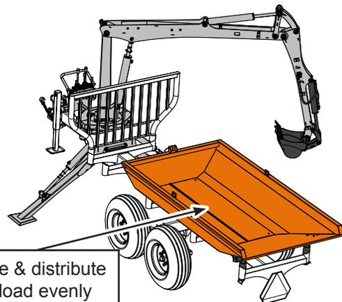
**⚠ Caution:** Ensure pivot tubes snap lock pins are in place to secure the dump box to the trailer.
