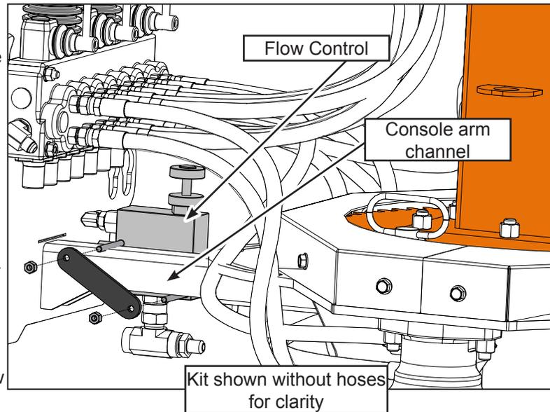
3. Review the hydraulic schematic, if you have a winch installed then **A** hose connection is switched with the hose connection at the return port of the winch hydraulic control.
