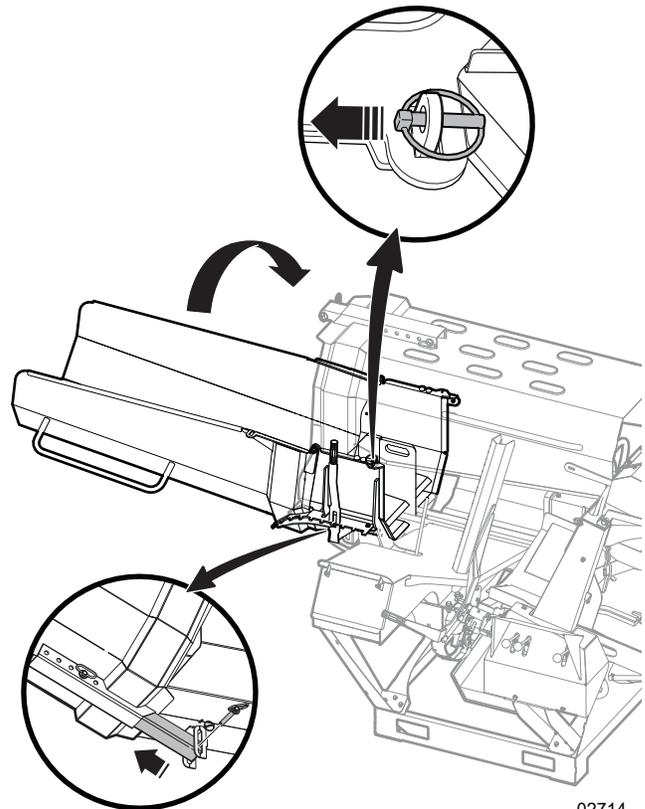
**Figure 41**—Fold the splitter chute
