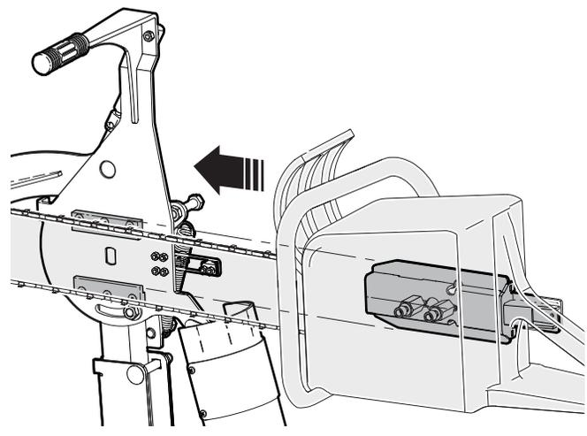
**Figure 32**—Put the chainsaw into the holder
