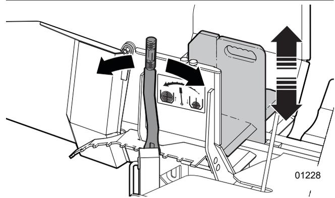
Figure 9—Splitting-wedge height adjustment
