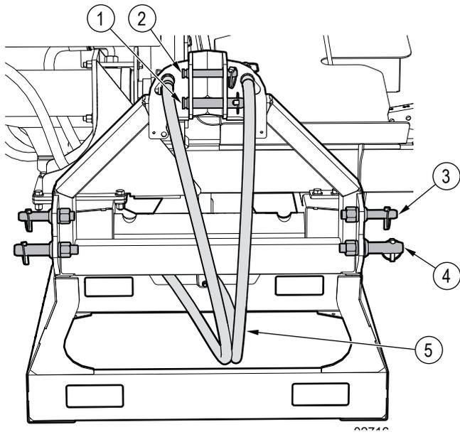
**Figure 44**—Machine three-point hitch connections
