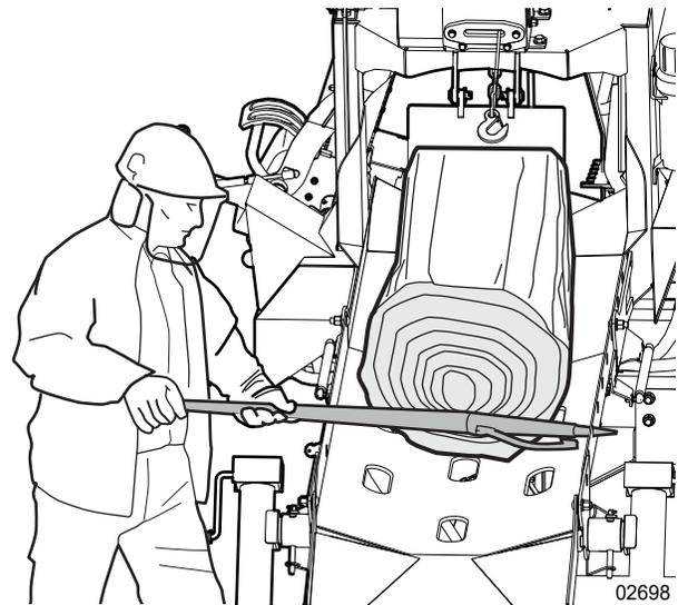
Figure 39—Use a tool to push the last log forward
