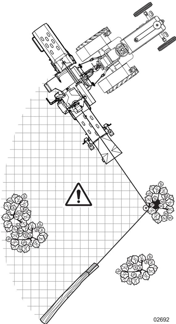
Figure 25—Example of how to use a snatch block
