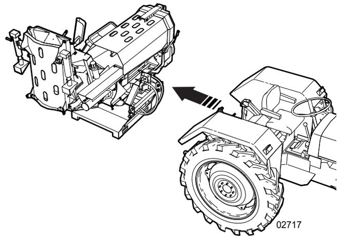
**Figure 45**—Align the tractor with the machine
