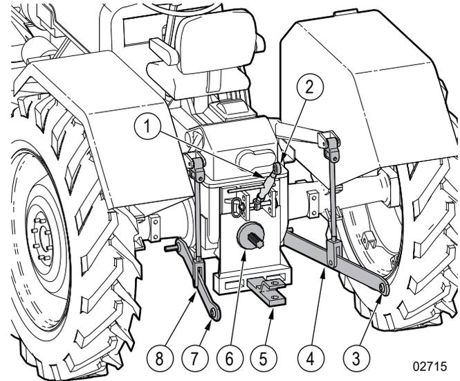
Figure 43—Tractor three-point hitch connections (example)
