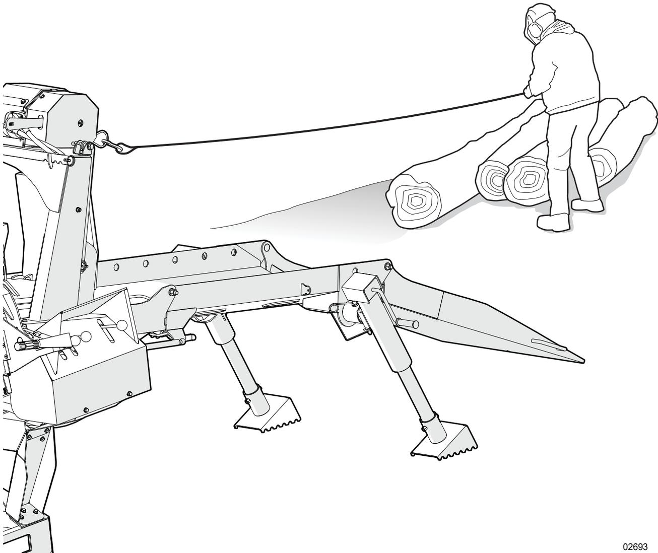
**Figure 28**–Pull the winch rope out to the log
