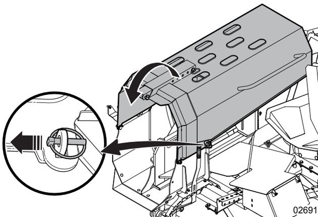
**Figure 16**—Splitter chute linchpin and latch tab
