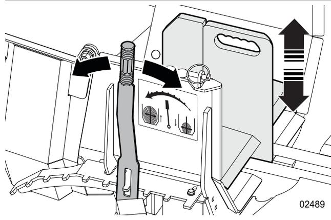
Figure 19—Set the splitting-wedge height
