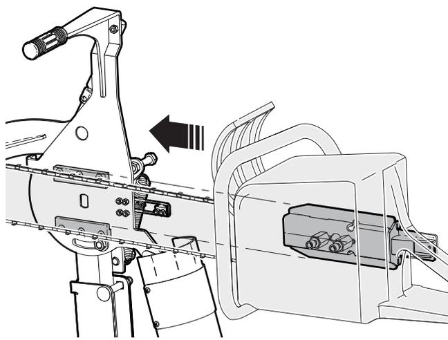
**Figure 23**—Put the chainsaw into the chainsaw holder
