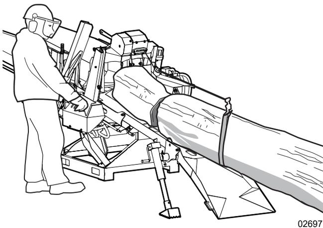
Figure 38—Use the next log to push the current log
