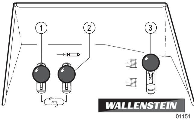
Figure 7—Hydraulic Controls
