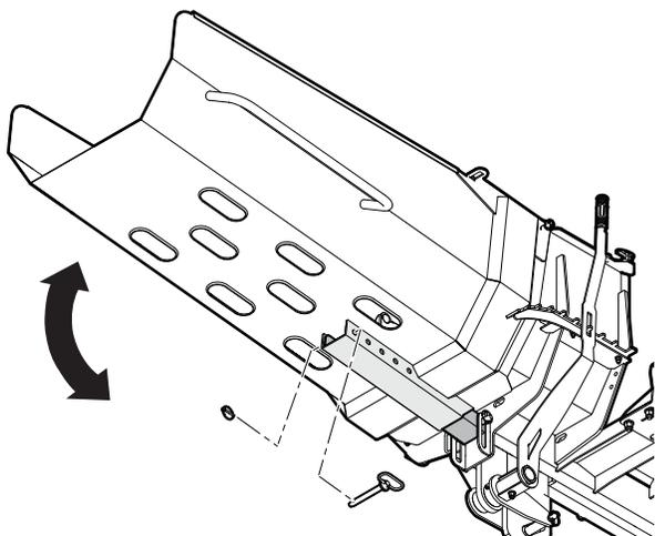
Figure 18—Set the splitter-chute height
