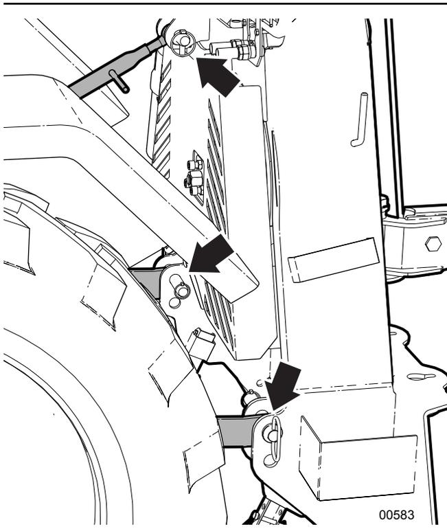
Fig. 8—Winch Attached
