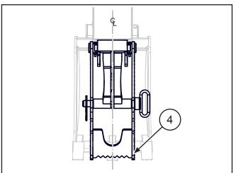
Fig. 3-Center thumb on dipperstick boom
