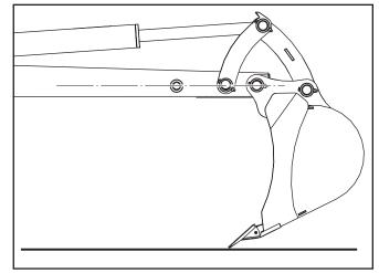
Fig. 1-Backhoe dipperstick boom horizontal
