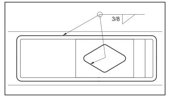
Fig. 4-Apply full weld around the plate
