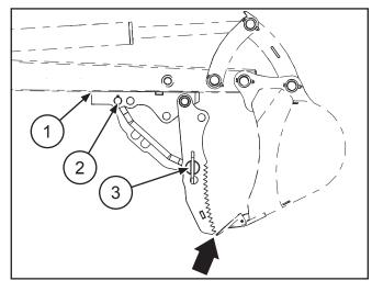
Fig. 2-Position thumb frame
