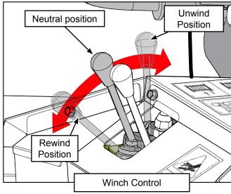
**Caution**: Always ensure the area is clear of bystanders when operating the winch, and never use the winch to hold or secure loads
