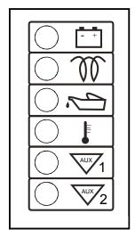
**Battery:** lights up when the ignition is set to "run", the indicator shuts off after the engine starts.
