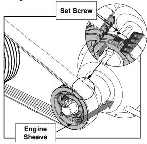
Note: movement of the sheave may occur when tightening the bushing, some allowance for movement may be required.
