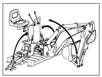
Carefully use the backhoe hydraulics to rotate the bracket assembly into the top attach points on the subframe. Rotate the bracket until it reaches the stop. The pin holes will then be aligned.
