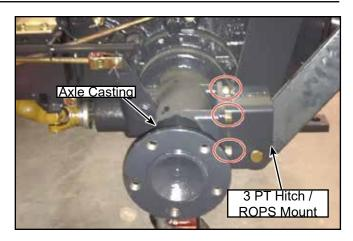
**Step 4** Remove the two bolts from the hitch left-hand side. Set bolts and washers aside.
