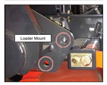
Place tractor weldment between the frame and ROPS mount. Leave loose for the next step.
