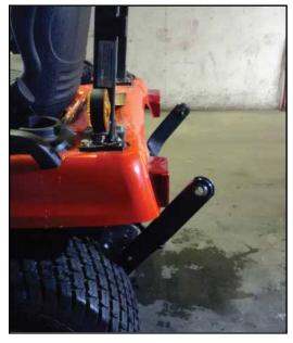
Remove three of the rear bolts of the frame, as shown for the left hand side in the image.
