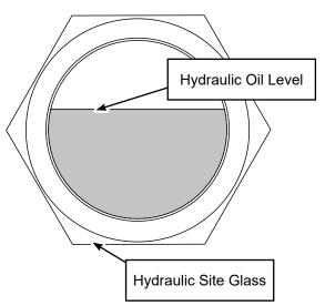
Hydraulic oil level should be checked daily, and the quality of the oil should be inspected every 50 hr. If the oil is dirty or smells burnt, it should be replaced.
