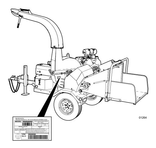
Fig. 1-Serial Number Plate Location
