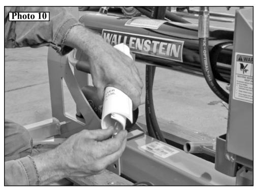
10. Secure all four (4) 1/2 X 5.5 Bolts using the supplied 1/2" Nylon Locknuts. *Photo* 11
