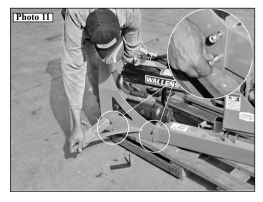
11. Snip Tie Wraps securing hydraulic hoses and lie out towards front of splitter for connection at tractor. *Photo 12 & (13 following Page)*
