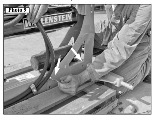
9. Locate plastic Manual Tube Cubby and remove two (2) more 1/2 x 5.5 Bolts and 1/2" Nylon Locknuts to be inserted into the two (2) remaining holes. *Photo 10*
