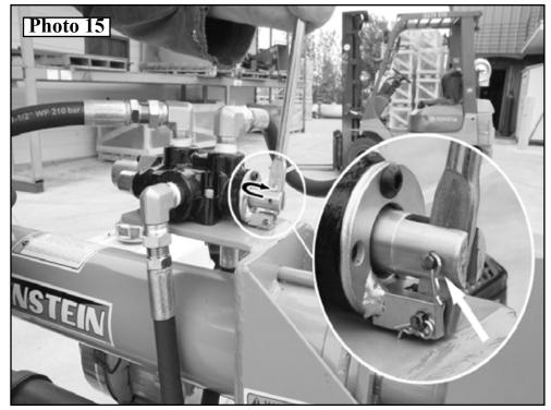
13. Install Handle in vertical position. Insert bottom slotted end of lever into lower pin aligning upper hole with one in shaft. *Photo 15* Install Pin and secure with Pin Clip. **See Photo Inset.**
