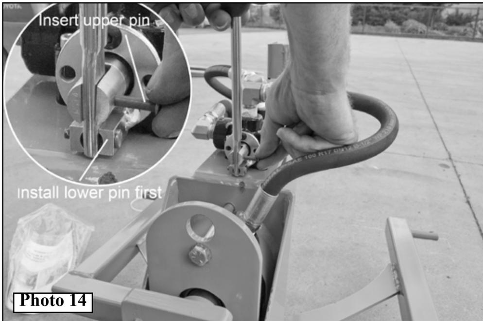
13. Insert upper pin and secure each pin with Pin Clip. **Photo 15**
