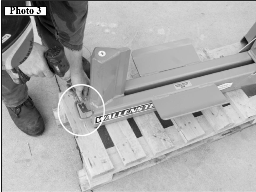
4. Remove mounting screw located on right hand side of splitter as illustrated in *Photo 4*
