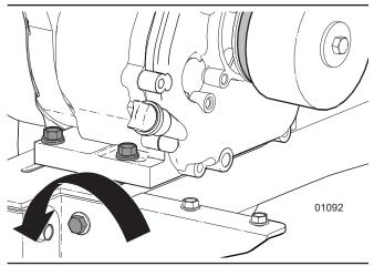
Figure 25-Rotor drive-belt tensioning bolt
