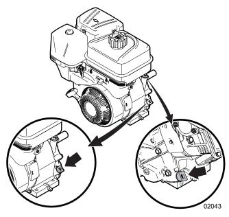
Figure 17 – Engine oil-fill locations
