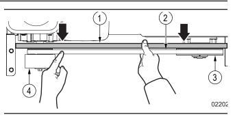
Figure 27 - Drive belt alignment
