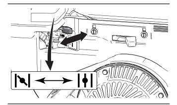
**Figure 9**—Engine choke control
