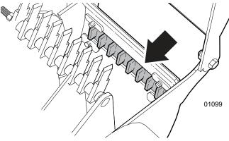
Figure 36-Chop Block in Rotor Housing
