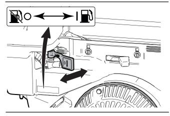
Figure 8-Engine fuel shutoff
