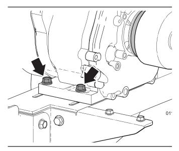
Figure 29 - Engine Mount Bolts
