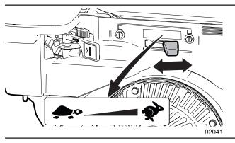
Figure 7—Engine throttle control
