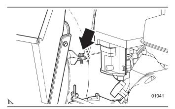
Figure 22-Upper rotor housing fastener
