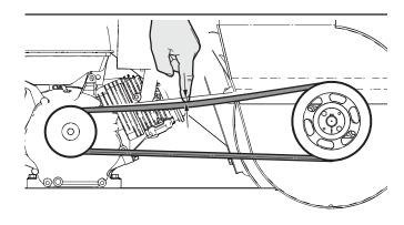
Figure 26 - Check the rotor drive-belt tension
