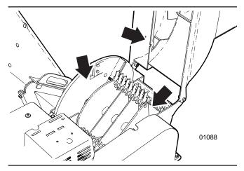
Figure 23 - Remove all material from the lower housing
