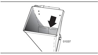
Figure 20 – Chipper hopper safety flap
