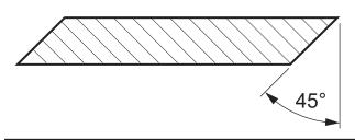
Figure 33 - Sharpen a rotor knife
