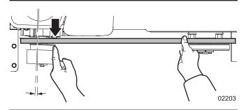
Figure 28-Engine mount alignment
