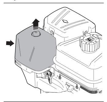
Figure 24-Remove the air filter
