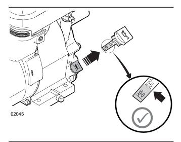
Figure 16-Check the engine oil level
