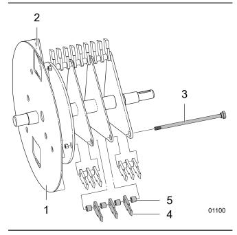
Figure 35-Rotor Assembly
