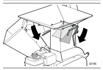
Figure 11 - Shredder gate levers
