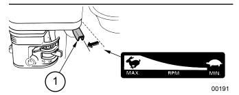
Fig. 20 - Engine Throttle
