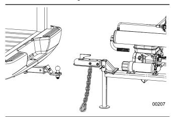
Fig. 29-Ball Hitch Aligned
