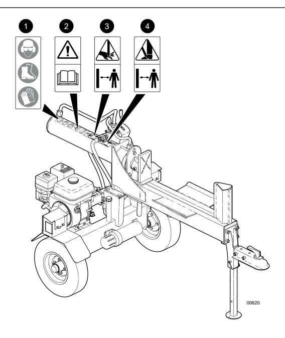
Fig. 2-Safety Decal Locations (typical for all WXR models)
