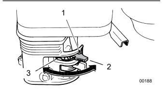
Fig. 7-Choke Lever
