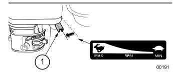
Fig. 9-Throttle Lever Positions
