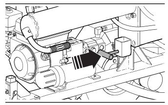
Fig. 27-Lock Pin Fully Engaged on WXR740 Series
