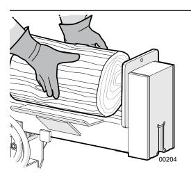
Fig. 23-Correct Log Placement
