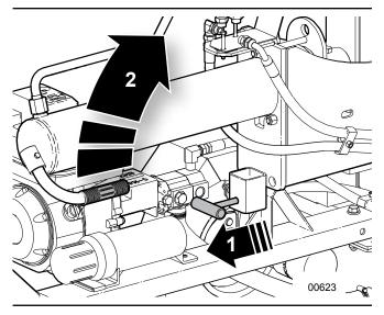
Fig. 18-Rotate Splitter to Vertical
