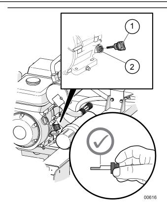
Fig. 12-Engine Oil Level check
