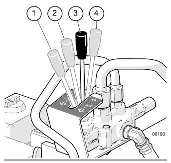
Fig. 11 - Hydraulic Control Valve Positions
