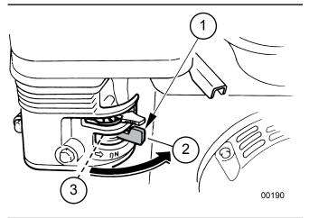
Fig. 8-Fuel Valve Lever
