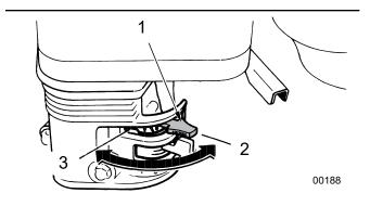
Fig. 19-Choke Lever
