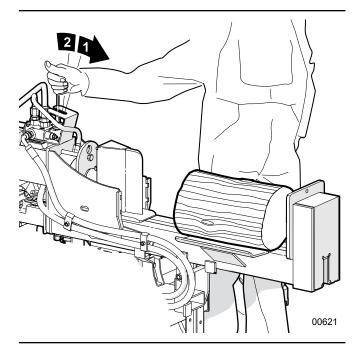
Fig. 25-High Speed (2), High Power (1)
