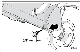
Fig. 31 - Hydraulic Tank Drain Plug
