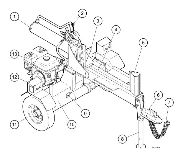
Fig. 3-WXR720, WXR720L Wood Splitter Components
