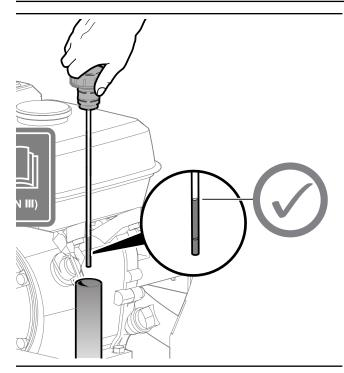
Fig. 13-Hydraulic Tank Oil Level Dipstick
