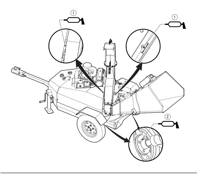
Figure 33 – Grease fitting locations
