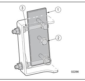
Figure 48-Ledger knife adjustment assembly (typical)
