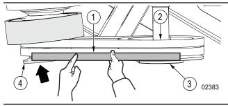
Figure 43 - Align the engine clutch
