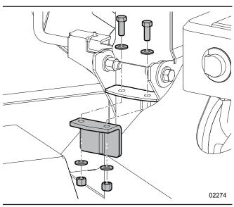
Figure 51 – Install a twig breaker
