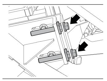
Figure 40 - Drive belt tensioning bolts
