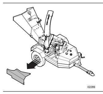
Figure 36-Remove the engine guard
