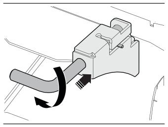
Figure 26 - Engage the rotor lock
