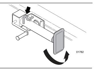
Figure 31 – Trailer jack in the stowed position
