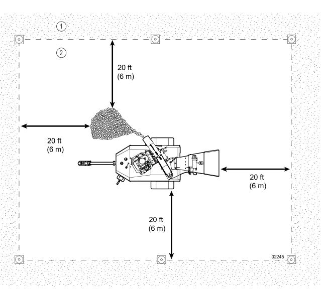
Figure 2-Example of a safe work area
