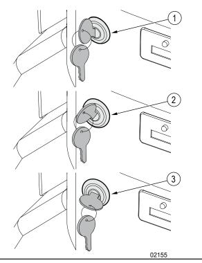
Figure 11 - Ignition switch positions
