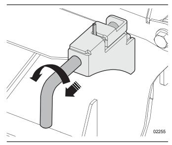
Figure 27 - Disengage the rotor lock
