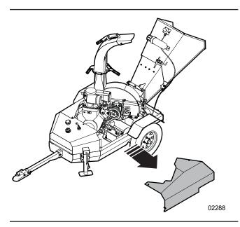
Figure 37 - Remove the drive-belt guard
