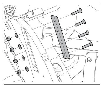
Figure 46-Install a rotor knife
