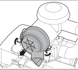
Figure 35-Remove the air-filter cover
