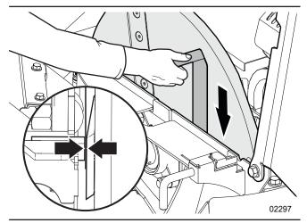
Figure 50 - Set the ledger knife clearance
