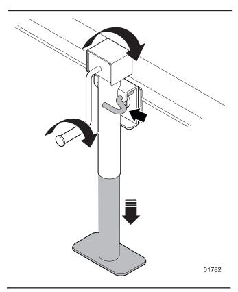
Figure 30 - Trailer jack in the lowered position
