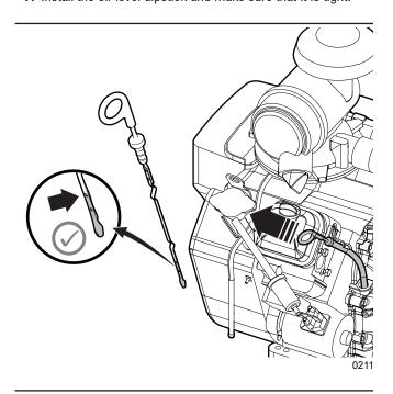
Figure 19 - Engine oil level check
