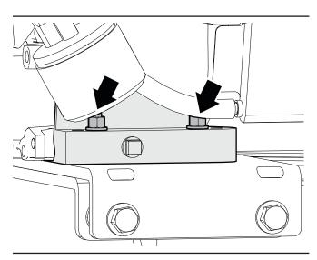
Figure 41 - Engine mount bolts (two of four)
