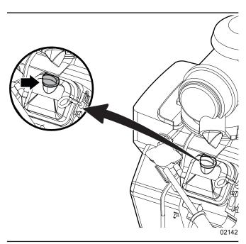
Figure 20 - Engine oil-fill location
