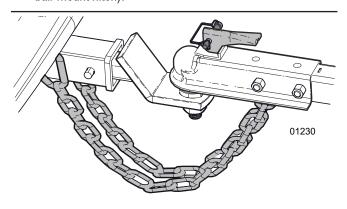
Figure 29 - Ball-mount hitch connection
