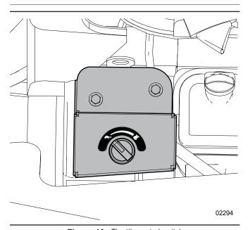
Figure 10 - Throttle control switch
