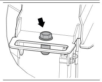
Figure 24-Upper-rotor-housing fastener
