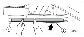
Figure 44 - Align the rotor sheave
