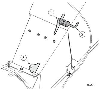
Figure 16-Chipper hopper latch
