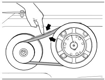
Figure 39 - Check the drive belt tension
