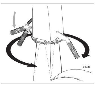
Figure 12 - Turn the discharge chute
