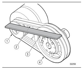
Figure 42 – Check the drive belt alignment
