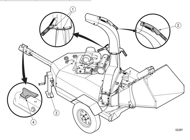
Figure 34 – Hinge and pivot point grease locations
