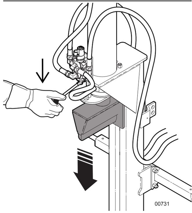
Fig. 5—Extend Wedge to split Wood
