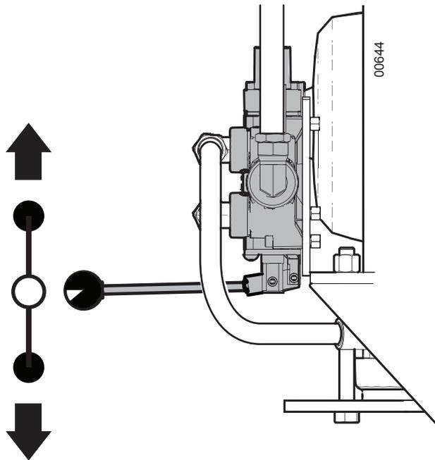
Fig. 4—Splitter Control Valve
