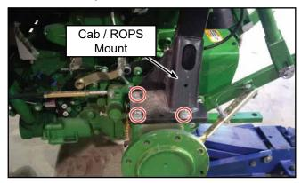
**4.** Remove the two bolts of the left-hand loader mount, as shown. Set the bolts aside.
