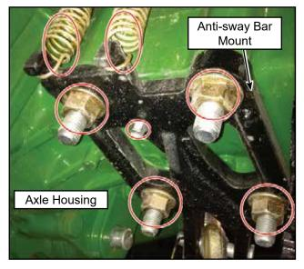
**3.** Remove the three of the through bolts from the cab/ROPS mount, as shown below for the left-hand side. Place the bolts in a safe place for later reuse.
