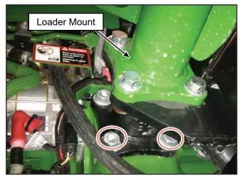
**5.** Remove the two bolts on the bottom of the hitch receiver, as shown. Set the bolts aside.
